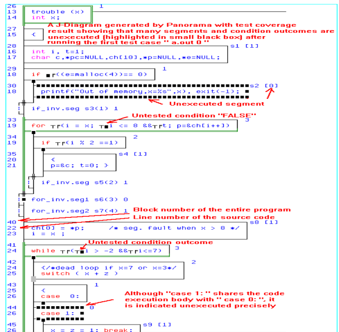
Fig. 30 The corresponding logic diagram shown in J-Diagram notation with untested branches and conditions highlighted in small black boxes
