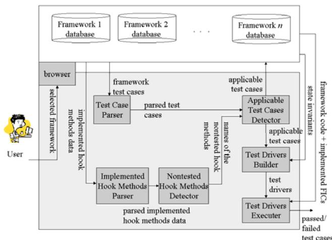
Fig. 8. Modified framework used part re-testing process
