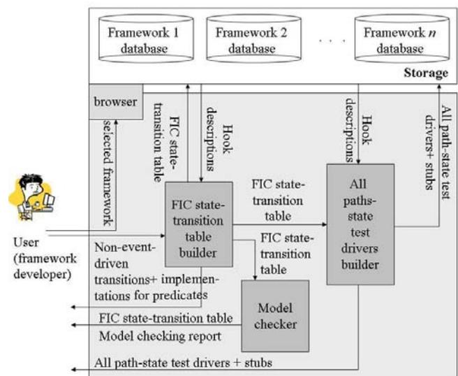
Fig. 9. The FIC test case generation process
