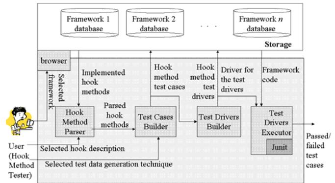
Fig. 7. Modified framework hooks testing process
