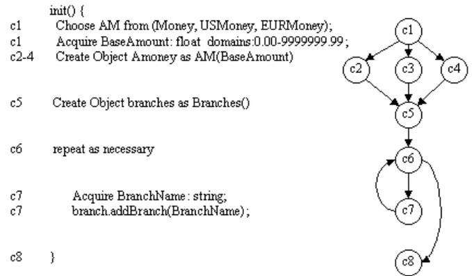
Fig. 5. The CFG of the *init()* method defined in the *Initialize Account* hook
