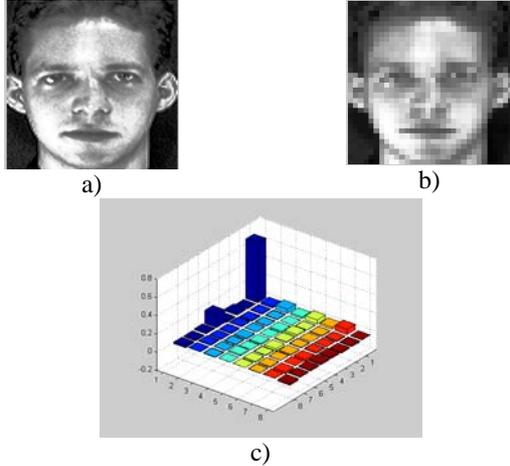
Fig. 7. a) Original image, b) Image with reduced pixel, c) DWT spectrum in a group of 8 x 8 pixels.
