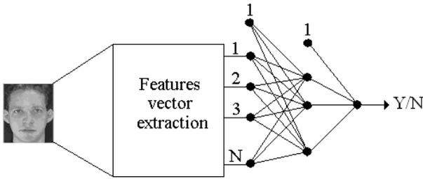
Fig. 2 Block diagram of proposed identity verification system,
