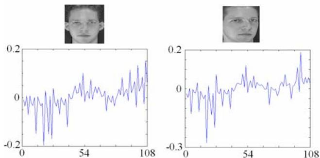
Fig. 17 Face images with different rotation and their feature vectors extracted using the discrete Walsh transform.
