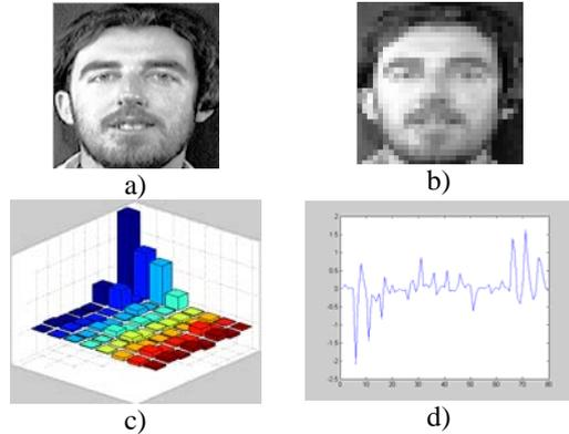
Fig. 8. a) Original image. b) Image with reduced pixel, c) DCT spectrum in a group of 8 x 8 pixels, d) Feature vector.
