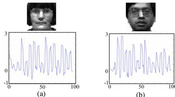
Fig. 20 Face images of two persons together with their feature vectors extracted using the discrete cosine transform.
