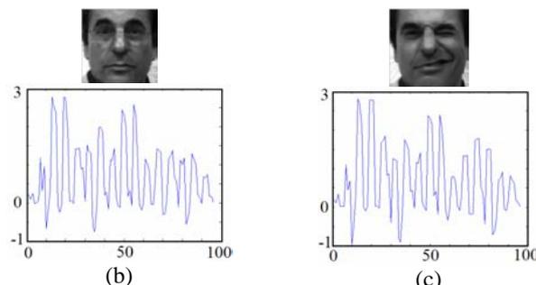
Fig. 19 Face images with different expressions and their feature vectors extracted using the discrete cosine transform.
