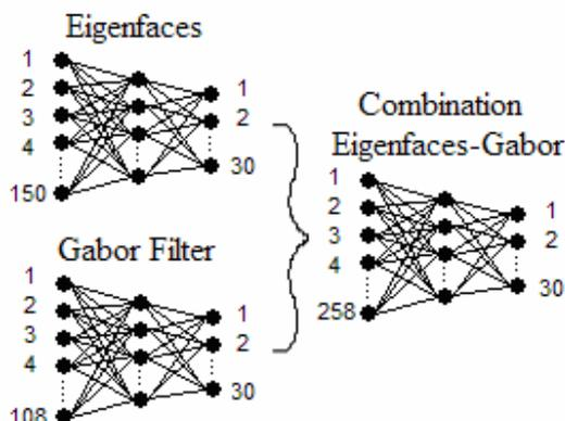
Fig. 21. Combination of Eigenfaces and Gabor in a neuronal network.
