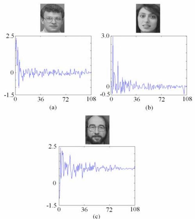
Fig. 16 Face images of several persons together with their feature vectors extracted using the eigenfaces method.
