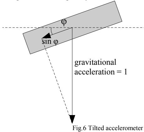
Fig.6 Tilted accelerometer
