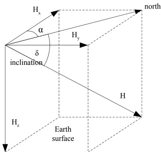
Fig.3 Earth's magnetic field vector in three dimensions.
