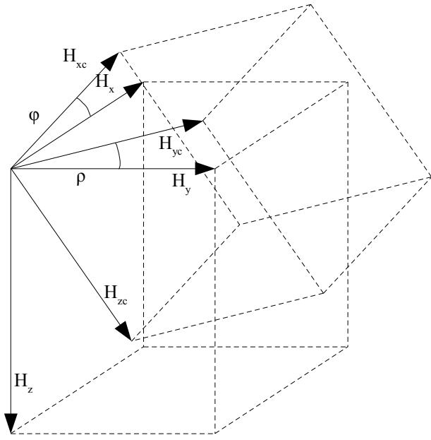
Fig.5 Components of Earth's magnetic field vector in different coordinate systems.
