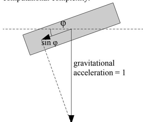
Fig.6 Tilted accelerometer
