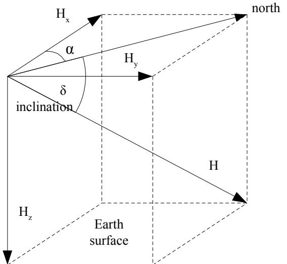
Fig.3 Earth's magnetic field vector in three dimensions.
