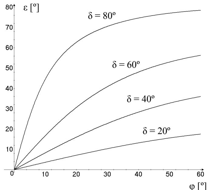
Fig.4 Error of determined azimuth, caused by compass rotation [8]
