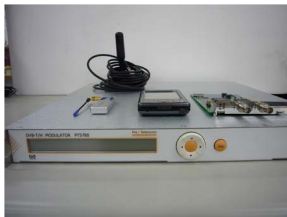
Fig. 12 Experimental hardware components and DVB-T/H modulator
