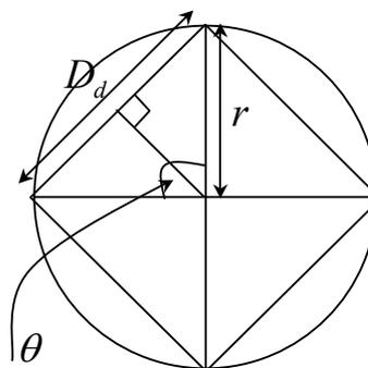
Fig. 9. Computing the radius of four robots circle.
