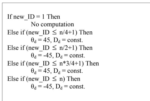
Fig. 11. Calculating the desired angle and distance for the leader for diamond formation.
