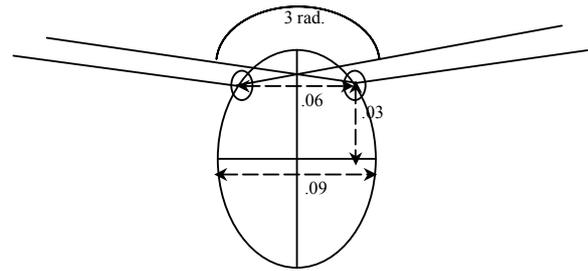
Fig. 2. The infrared eye mechanism (all units in meters).
