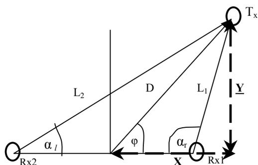
Fig. 7. Calculating the distance and angle of a friend robot.
