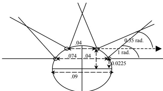
Fig. 1. Collision avoidance sensors arrangement (all units in meters).
