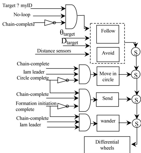
Fig. 4. The proposed robot behaviors and their interaction.
