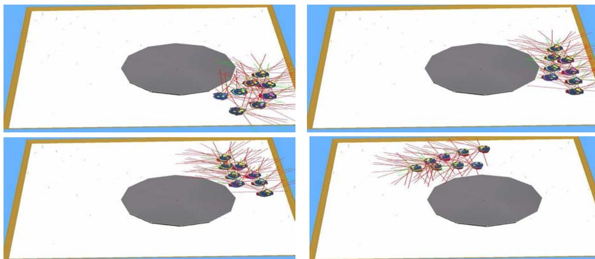
Fig. 15. Formation shrinks during the passage through narrow corridors (wedge).
