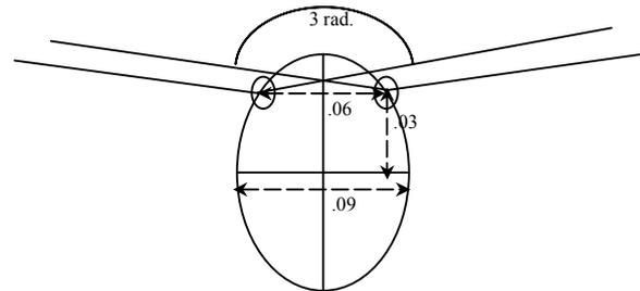
Fig. 2. The infrared eye mechanism (all units in meters).
