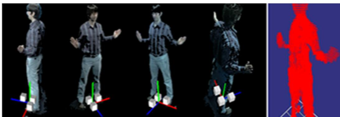
Fig. 8: On the left, the projected subject silhouettes obtained from four different points of view, and on the right its corresponding 3D shape reconstruction.
