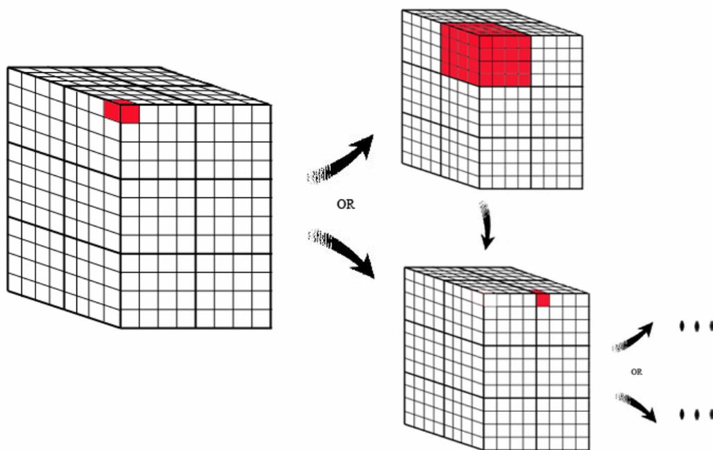
Fig.7: The BAVC algorithm step by step. Firstly, it starts checking one voxel, and depending how it is labelled the procedure follows by checking the neighbors or, by checking the next voxel with a step S.
