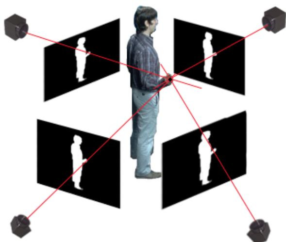
Fig. 1: An example of how the rays intersect in the hand of the subject. Each ray starts from the camera center, and crosses its corresponding image silhouette.
