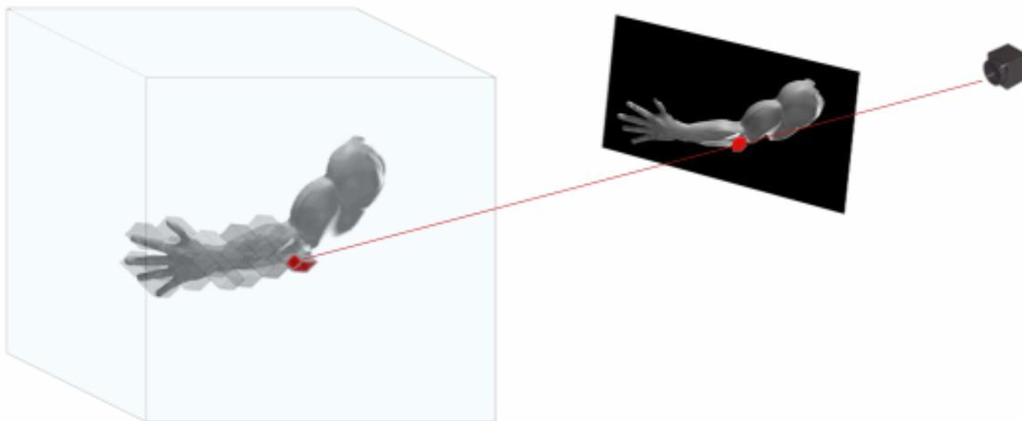
Fig. 3: A voxel carving method is being computed to the forearm checking Only the occupancy of the voxel's center [26]. The ray crosses a silhouette edge from the camera viewpoint and goes into the bounding volume.
