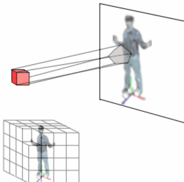
Fig. 2: An example of how the bounding volume is discretized into cubes with the same size and how on of these is projected into one of the silhouettes.
