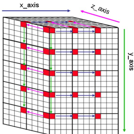
Fig. 6: The grid of voxels is tested with a step value of 4. The boundaries of the checked voxel neighborhoods are outlined with rough lines.
