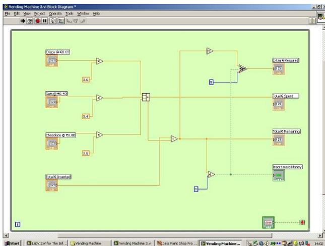
Fig.10 Block Diagram of Vending Machine
