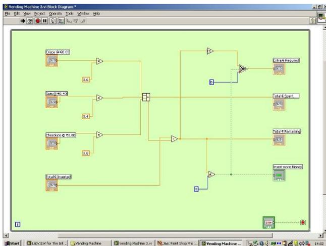
Fig.10 Block Diagram of Vending Machine
