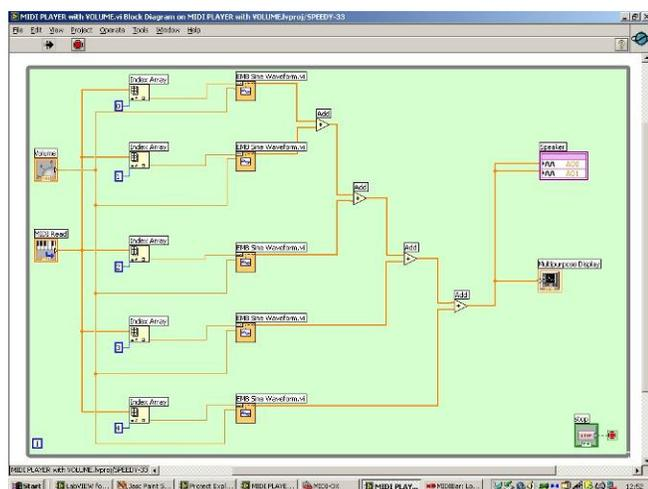
Fig.5 Block Diagram of Completed MIDI Player
