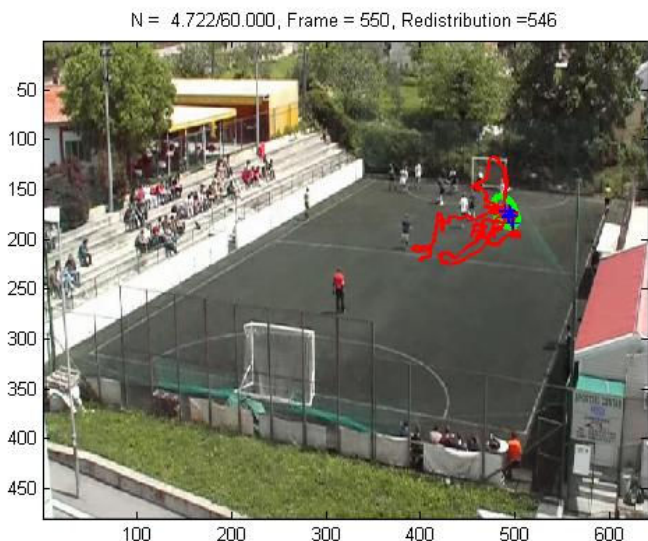
Fig. 4 Boosted particle filter tracking
