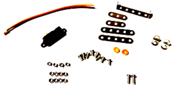
Fig. 19 a) – Sensor and components of Merkur building kit
