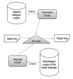
Fig. 2. An architecture example of a statistical machine translation system
