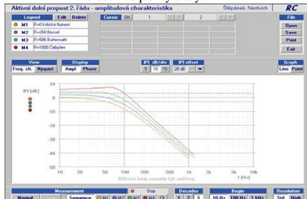
Fig. 4 Measured characteristics lowpass 2nd order - frequency analysis
