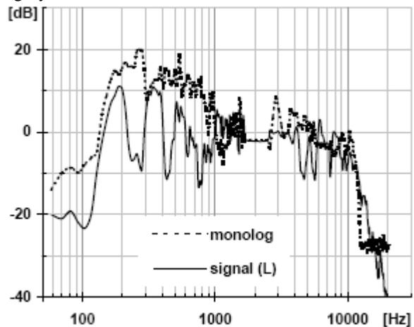
Fig. 8 Comparing the spectra of female voices from logatomic tests and monologues
