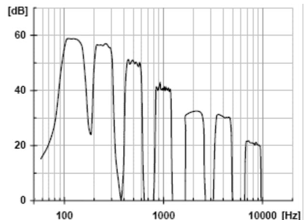
Fig. 5 Spectrum of STIPA signal (S)
