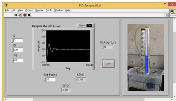
Fig. 27 Level System response with a PID controller ( $K_p = 5$ ,  $K_i = 0.25$ ,  $K_d = 0.1$  and Set Point = 20.)
