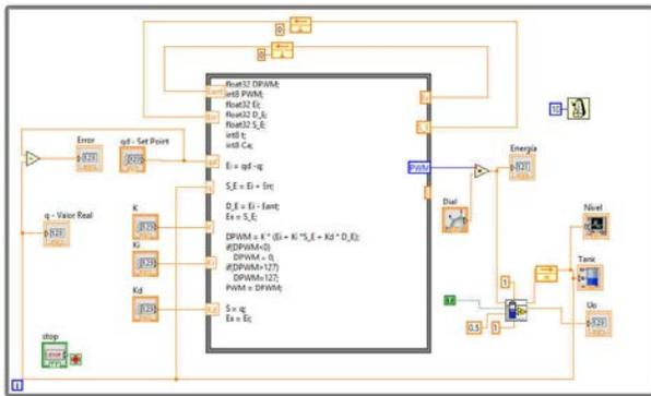
Fig. 23 Block Diagram of the PID controller
