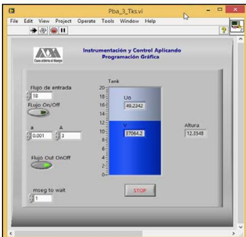
Fig. 8 Level System simulation
