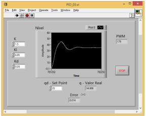
Fig. 20. Level System response with a PID controller  $(K_p = 1.5, K_i = 0.05 \text{ and } K_d = 0.05.)$
