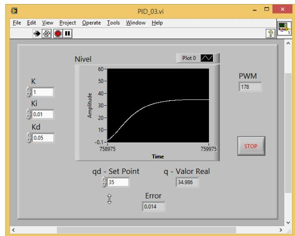
Fig. 22 Level System response with a PID controller ( $K_p = 1$ ,  $K_i = 0.1$  and  $K_d = 0.5$ .)
