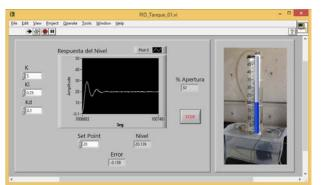
Fig. 27 Level System response with a PID controller  $(K_p = 5, K_i = 0.25, K_d = 0.1 \text{ and Set Point} = 20.)$
