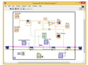
Fig. 16 Block diagram of the Level Control System with hysteresis of two tanks
