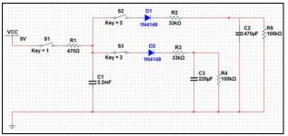
Fig. 17 Diagram of the RC circuit to emulate the three tanks system
