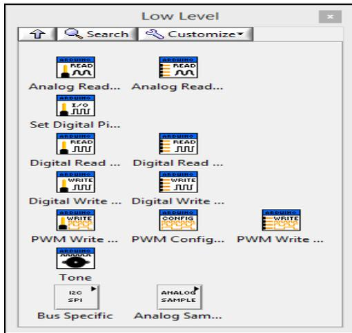
Fig. 12 Arduino communication toolbox
