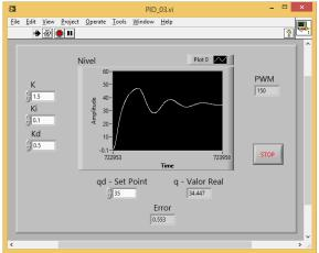
Fig. 21 Level System response with a PID controller  $(K_p=1.5, K_i=0.1 \text{ and } K_d=0.5.)$
