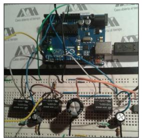
Fig. 18 Actual diagram of the RC circuit to emulate the three tanks system
