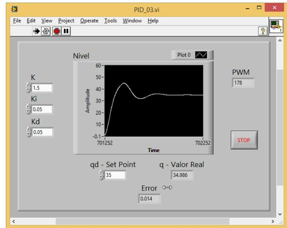
Fig. 20. Level System response with a PID controller ( $K_p = 1.5$ ,  $K_i = 0.05$  and  $K_d = 0.05$ .)
