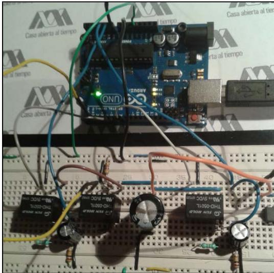
Fig. 18 Actual diagram of the RC circuit to emulate the three tanks system
