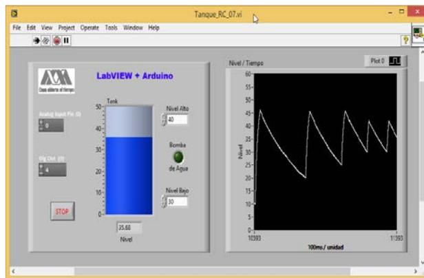
Fig. 15 VI using a RC circuit and Arduino with different control limits and hysteresis
