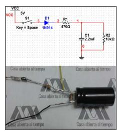
Fig. 13 RC Simulation of a Level System with output flow
