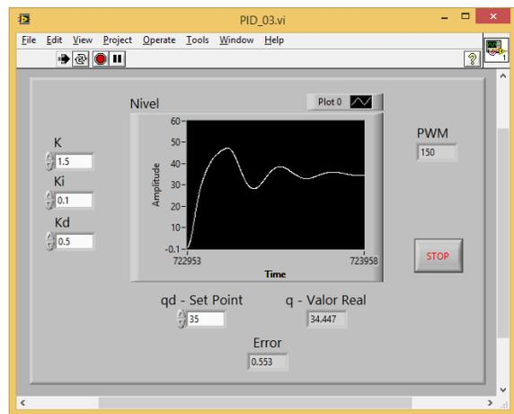
Fig. 21 Level System response with a PID controller ( $K_p = 1.5$ ,  $K_i = 0.1$  and  $K_d = 0.5$ .)
