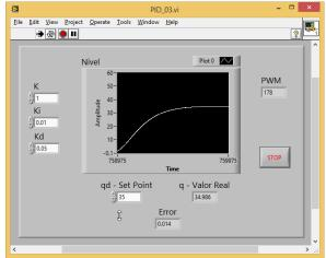
Fig. 22 Level System response with a PID controller  $(K_p=1,\,K_i=0.1 \text{ and } K_d=0.5.)$
