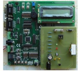
Fig. 3 Evaluation kit with Freescale HCS08GB60 microcontroller and model of heat plant
