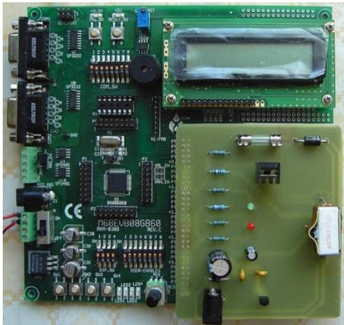
Fig. 3 Evaluation kit with Freescale HCS08GB60 microcontroller and model of heat plant
