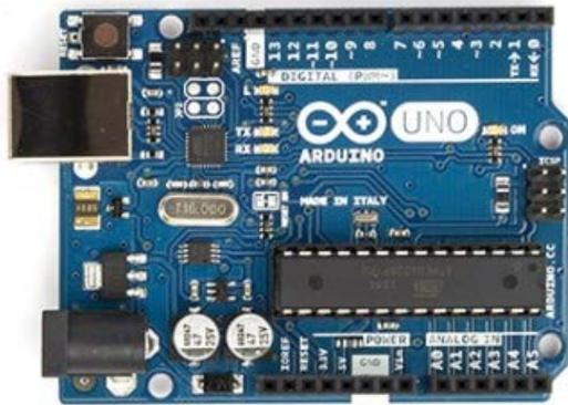
Fig. 5 Arduino Uno board [1]
