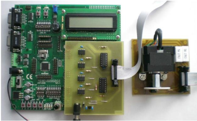
Fig. 2 Evaluation kit with Freescale HCS08GB60 microcontroller and external module with stepper motor
