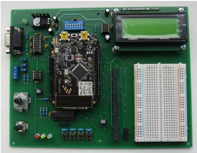
Fig. 7 Prototype of the kit; FRDM-KL25Z board attached
