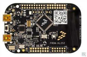
Fig. 4 Freescale FRDM-KL25Z board used in the kit [7]
