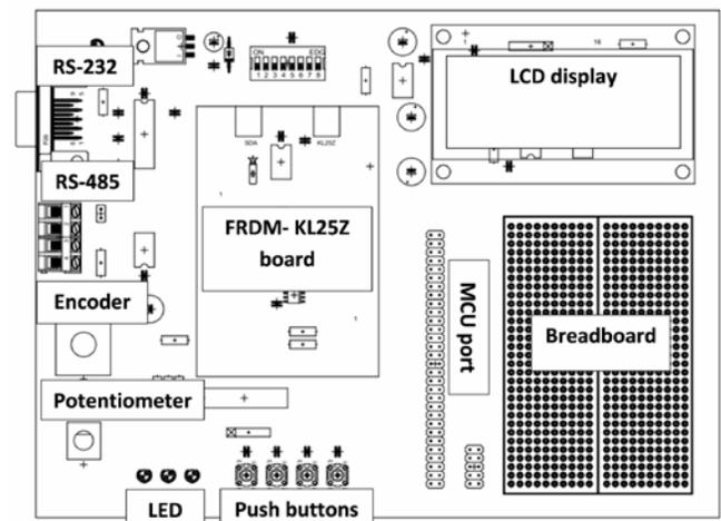
Fig. 6 Layout of the peripherals of the new kit
