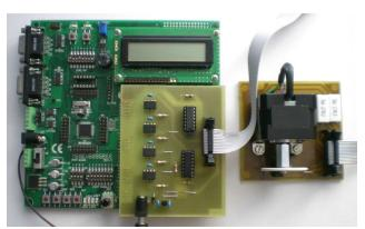
Fig. 2 Evaluation kit with Freescale HCS08GB60 microcontroller and external module with stepper motor
