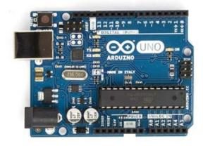
Fig. 5 Arduino Uno board [1]
