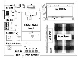
Fig. 6 Layout of the peripherals of the new kit
