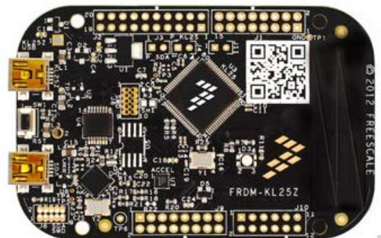
Fig. 4 Freescale FRDM-KL25Z board used in the kit [7]
