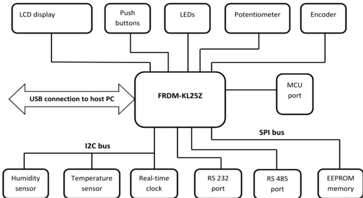
Fig. 8 Main components of the new kit based on FRDM-KL25Z
