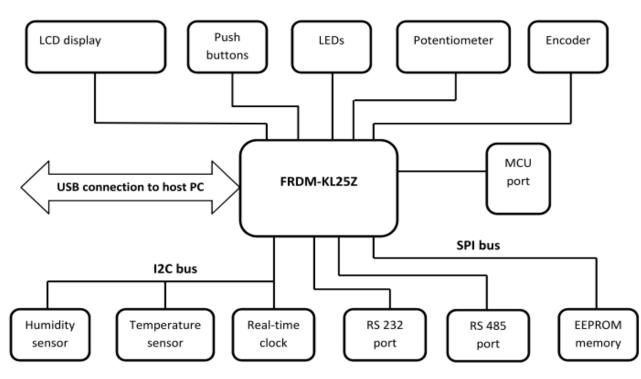
Fig. 8 Main components of the new kit based on FRDM-KL25Z
