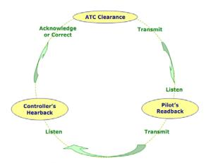
Fig. 3 The pilot – controller communication loop [7].
