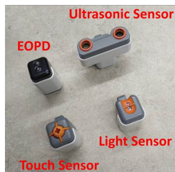
Fig. 4 Different types of sensors used in the construction
