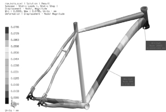
Fig. 8 3D virtual prototype of a mountain bike frame.
