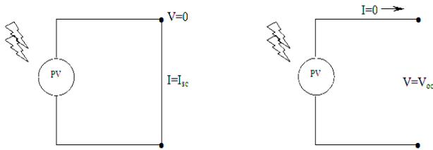
(a) Short-circuit current (b) Open-circuit voltage
