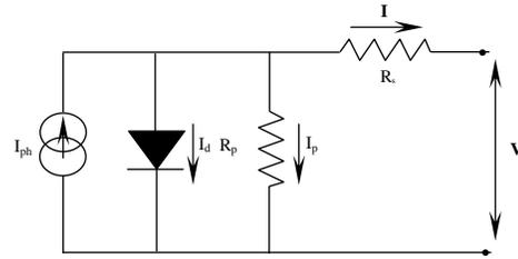
Fig. 3 the circuit diagram of the PV model.
