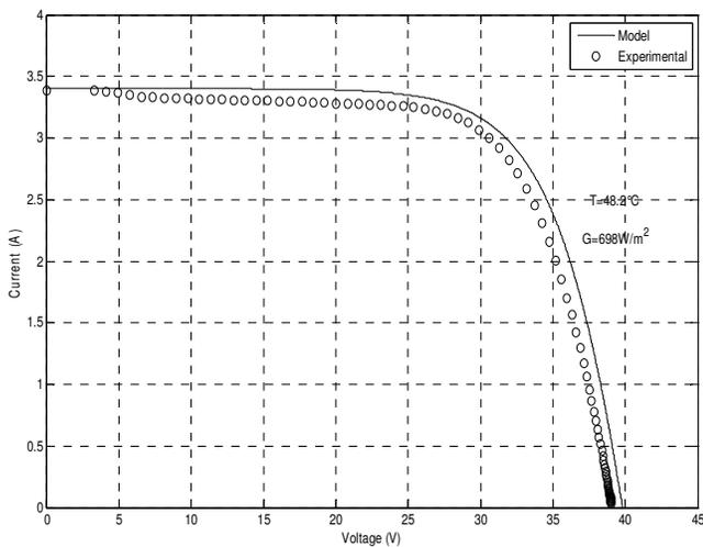
Fig. 12.a I-V characteristics of PV module (numerical simulation results with experimental data)
