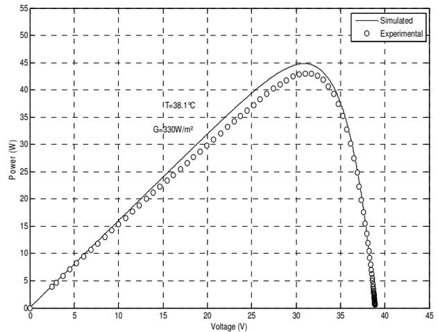
Fig. 10.b P-V characteristics of PV module (numerical simulation results with experimental data), for T=38.1°C, G=330W/m<sup>2</sup>
