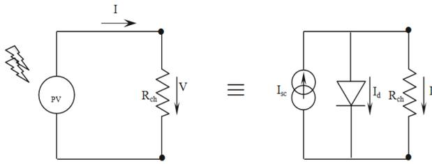
Fig. 4 PV cell with a load and its simple equivalent circuit
