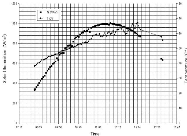
Fig. 2 the curves of temperature and irradiance versus time
