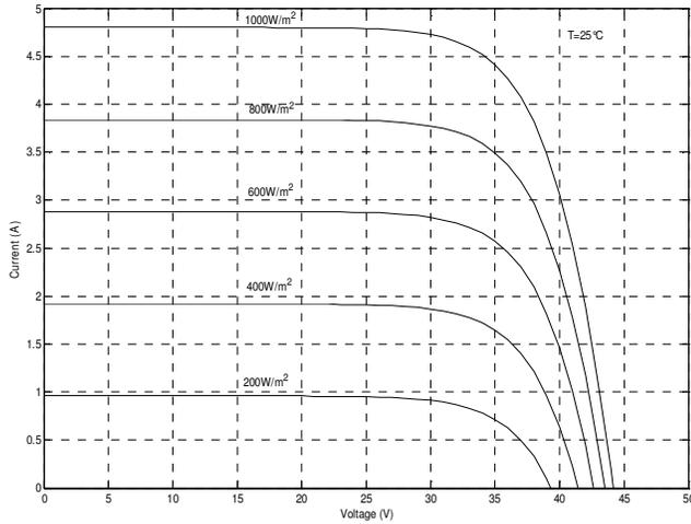
Fig. 8 Simulated I-V curves of PV module influenced by solar illumination
