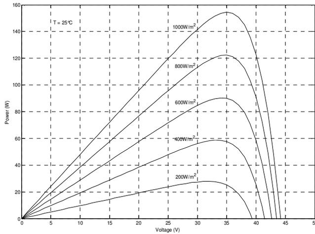
Fig. 9 Effect of illumination on the characteristic P-V of PV module at T = constant.
