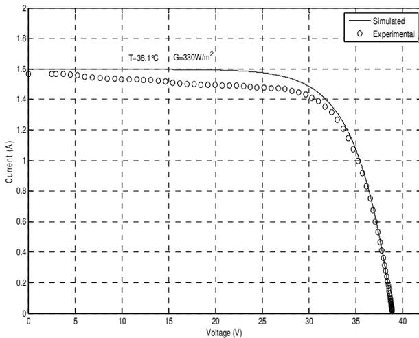
Fig. 10.a I-V characteristics of PV module (numerical simulation results with experimental data)
