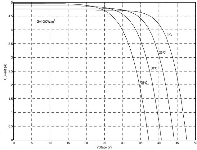
Fig. 6 Simulated I-V curves of PV module influenced by temperature at  $G=$  constant
