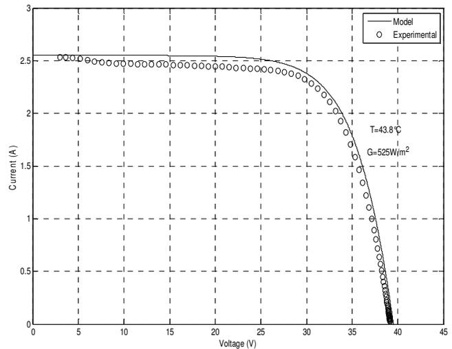
Fig. 11.a I-V characteristics of PV module (numerical simulation results with experimental data)
