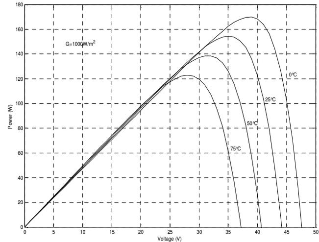
Fig. 7 Effect of temperature on the characteristic P-V of PV module at  $G =$  constant
