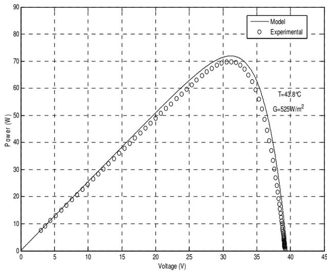
Fig. 11.b P-V characteristics of PV module (numerical simulation results with experimental data)
