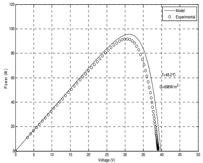
Fig. 12.b P-V characteristics of PV module (numerical simulation results with experimental data)
