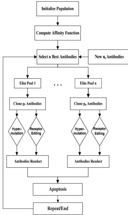
Fig. 6. Flowchart of Clonal Selection Algorithm
