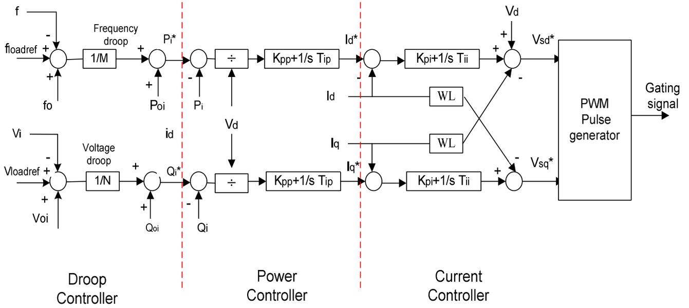
Fig. 2. Control Block Diagram for Interface Inverter[18]
