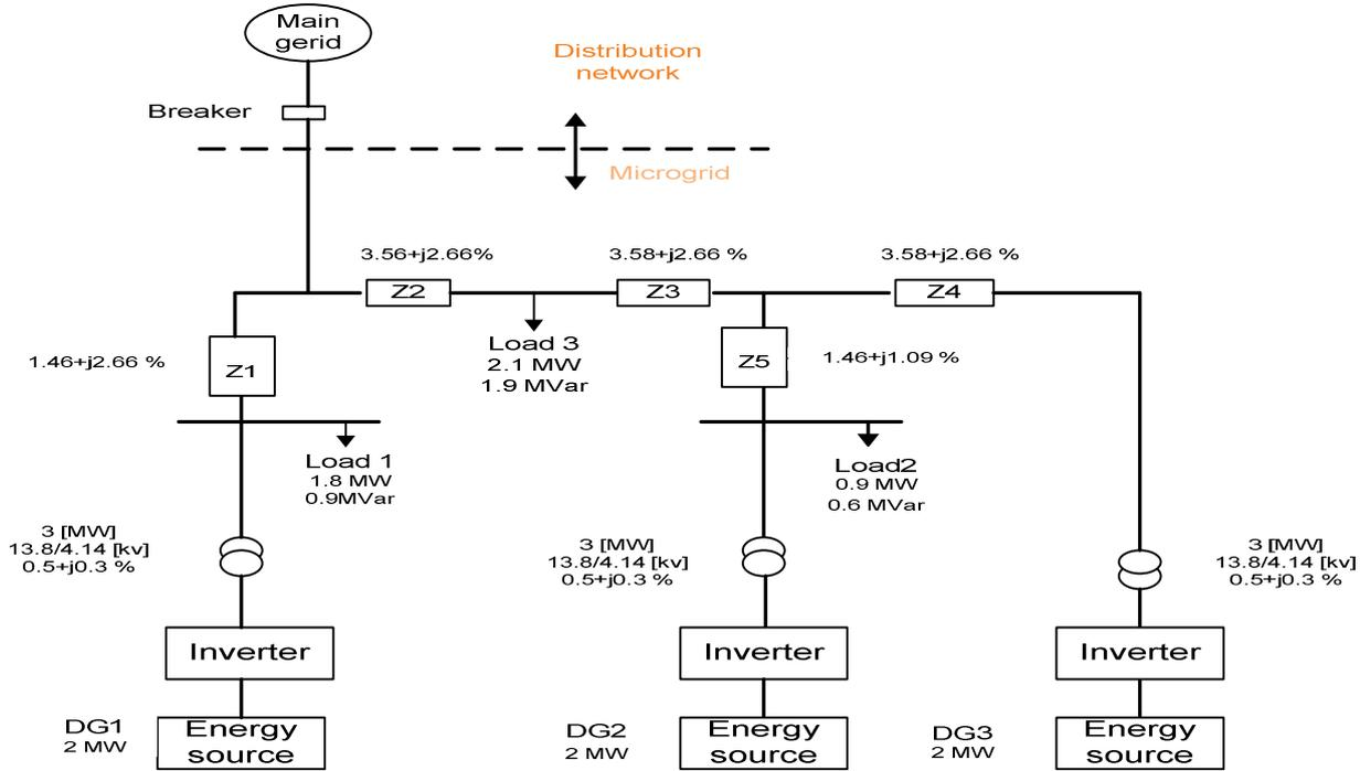
Fig. 1. Single Line Diagram of Microgrid
