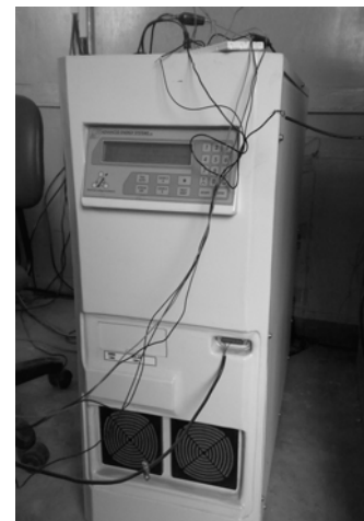
Fig. 3 Hybrid Inverter System
