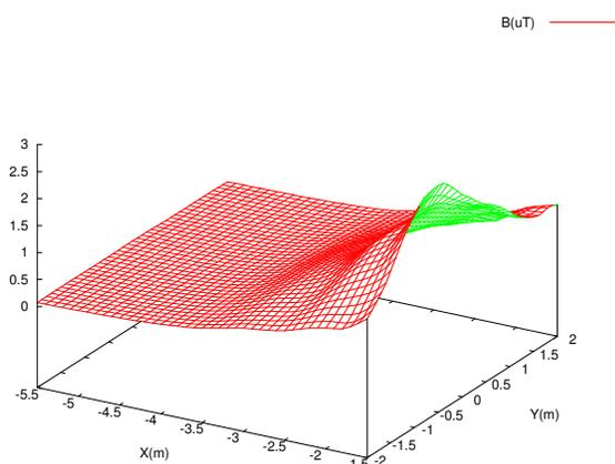
Figure 17: Section of the flux density approximation – Substation Podi 9 - Western side
