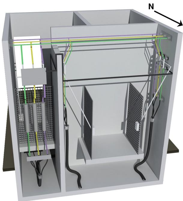
Figure 3: Layout of urban power substation Škrape 10 - northern side
