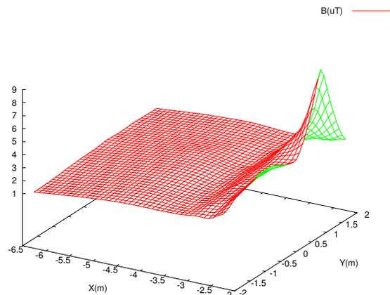
Figure 13: Section of the flux density approximation – Substation Škrabe 10 - Western side
