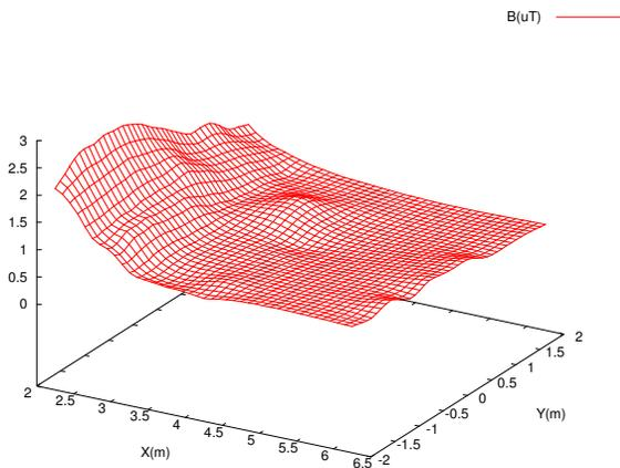
Figure 11: Section of the flux density approximation – Substation Škrabe 10 – Eastern side
