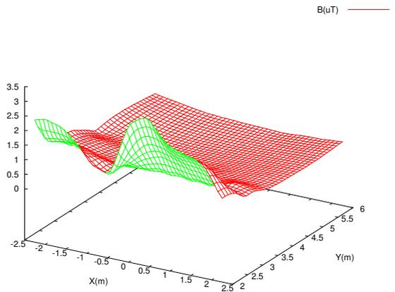
Figure 12: Section of the flux density approximation – Substation Škrabe 10 - Northern side
