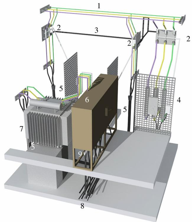
Figure 1: Equipment of urban power substation Škrape 10
