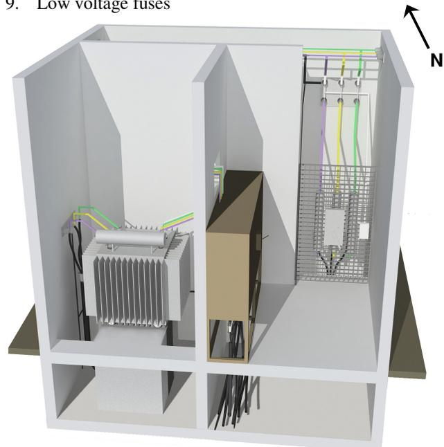
Figure 2: Layout of urban power substation Škrape 10 – southern side
