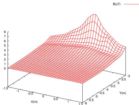
Figure 14: Section of the flux density approximation – Substation Podi 9 - Southern side
