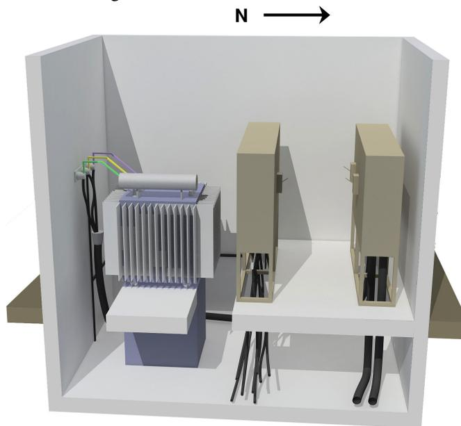
Figure 6: Layout of urban power substation Podi 9– eastern side
