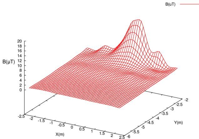
Figure 10: Section of the flux density approximation – Substation Škrabe 10 - Southern side
