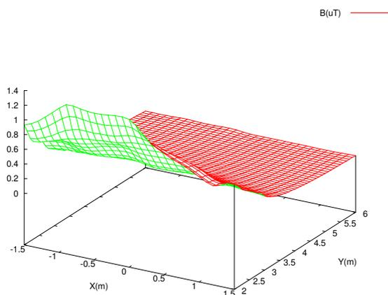
Figure 16: Section of the flux density approximation – Substation Podi 9 - Northern side
