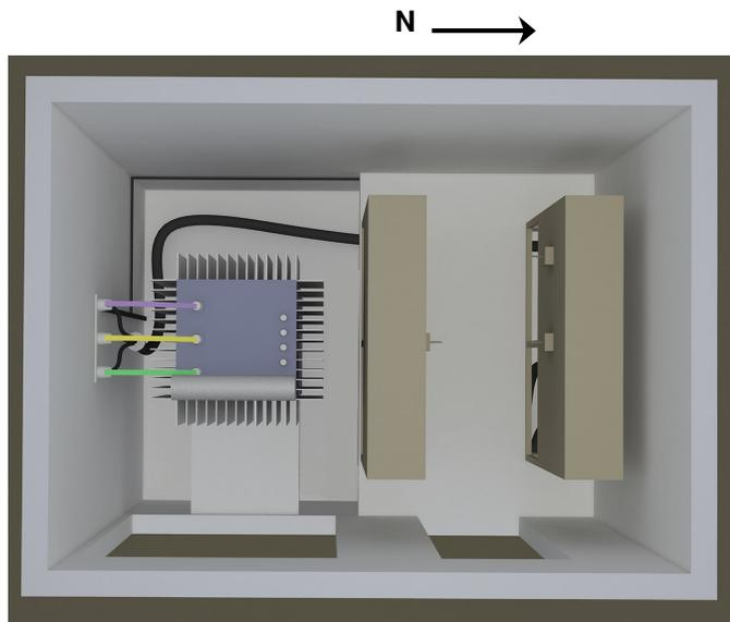
Figure 7: Layout of urban power substation Podi 9– top view
