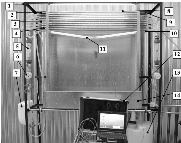
1) base frame, 2) temperature measurement of inlet falling fluid, 3) testing tube bundle, 5) flow meter, 6) integration flow meter, 7) heater
