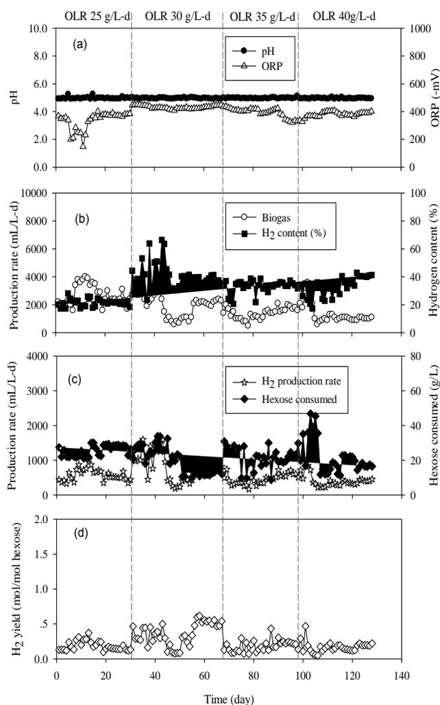
Fig.2 Performance of ASBR (a) pH and ORP, (b) biogas and hydrogen content, (c) hydrogen production rate and hexose consumed and (d) hydrogen yield.
