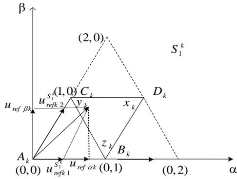
Fig. 3 First sector corresponding to the space voltage vectors of a three-level inverter.
