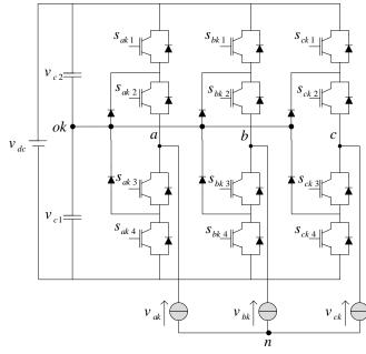
Fig. 1 Three-level inverter (k = 1 for first inverter and k = 2 for second inverter).
