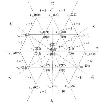
Fig. 2 Space vector diagram showing switching states for a threelevel inverter.
