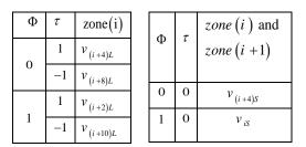
Table 3. First star switching table used in the conventional DTC.
