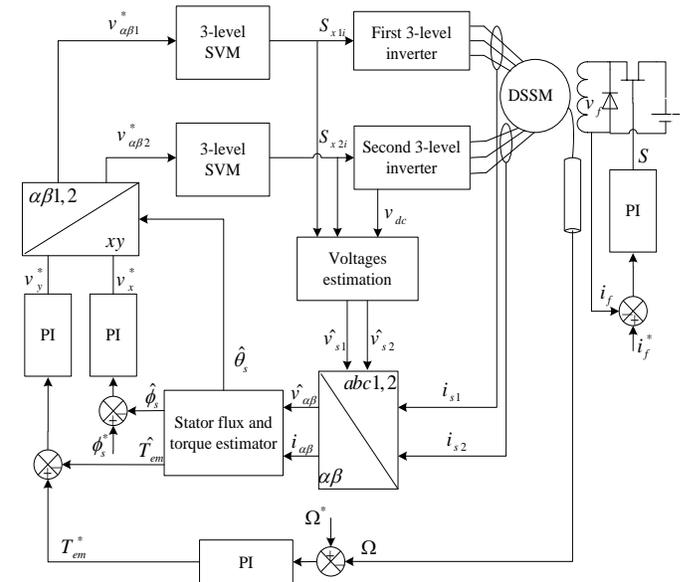
Fig. 6 DTC-SVM of DSSM (with  $j=1, 2, 3$  or  $4$ ).
