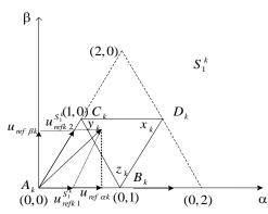
Fig. 3 First sector corresponding to the space voltage vectors of a three-level inverter.
