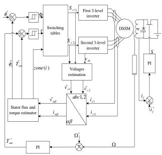
Fig. 5 DTC scheme for DSSM (with j=1, 2, 3 or 4).
