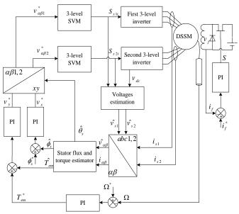
Fig. 6 DTC-SVM of DSSM (with *j*=1, 2, 3 or 4).
