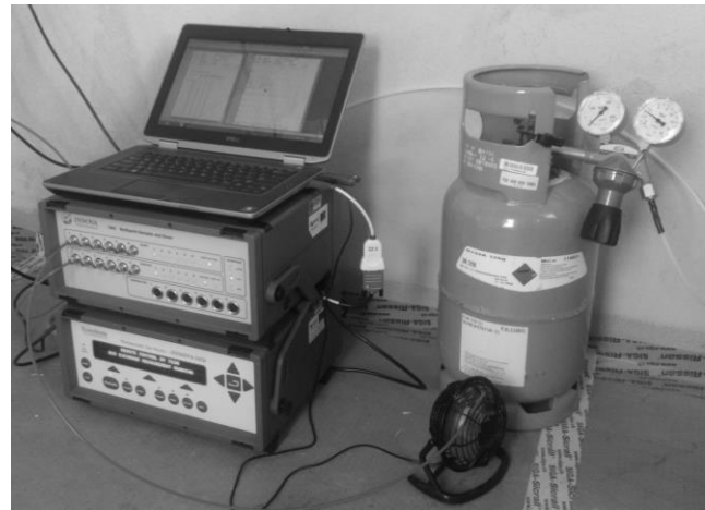
Fig. 5. System used for tracer gas air exchange measurements.
