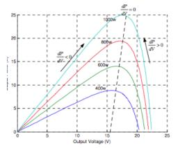
Fig. 4 – PV array characteristic
