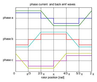
Fig. 1 – Phase currents and back EMF waves of a PM brushless dc machine
