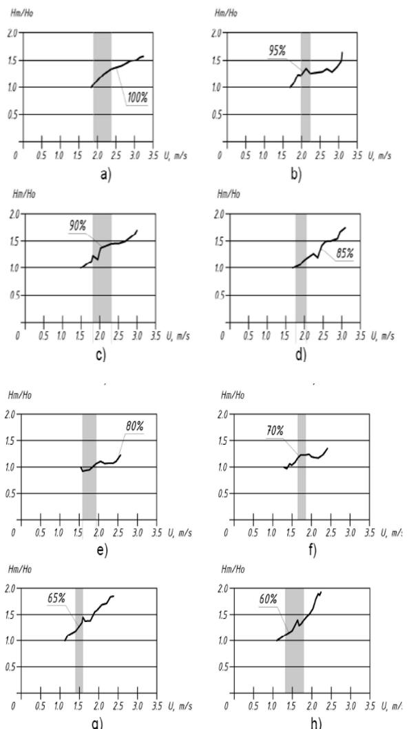
Fig 8 (a-h). Relative height of a bed vs. airflow rate for different mixtures. Diagrams show the content of straw pellets in a bed.
