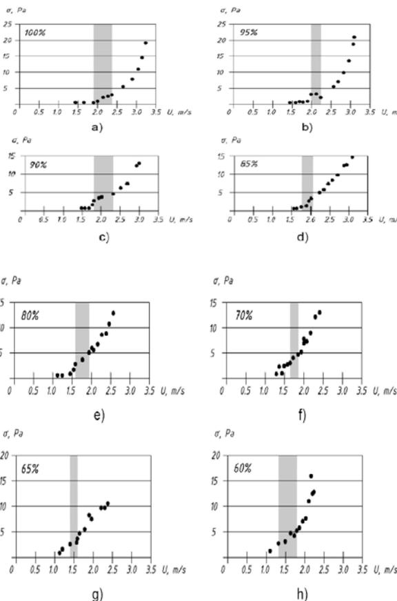
Fig 7 (a-h). Root-mean-square deviation of pressure fluctuations vs. airflow rate for different mixtures. Diagrams show the content of straw pellets in a bed.
