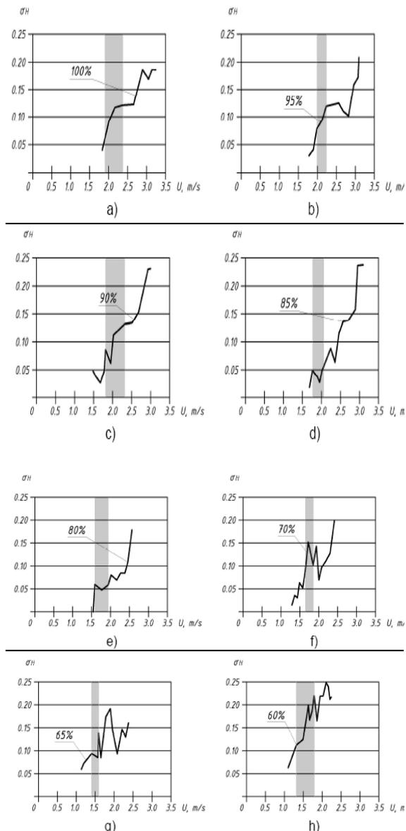
Fig 9 (a-h). Root-mean-square deviation of a bed relative height value vs. average value of airflow rate for different mixtures. Diagrams show the content of straw pellets in a bed.
