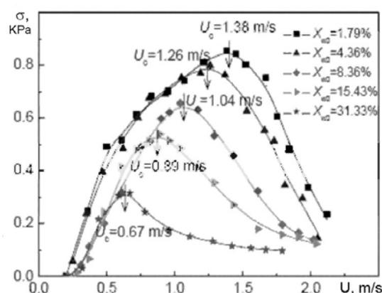
Fig 1. Standard deviation of pressure drop in a bed vs. airflow rate blown through a bed of sand and biomass pieces
