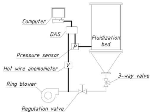
Fig 5. Schematic diagram of the experimental unit.
