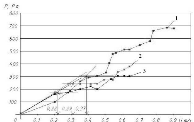
Fig 3. Curves obtained in the study of fluidization process of sawdust (1), rice husks (2) and nut shells (3).
