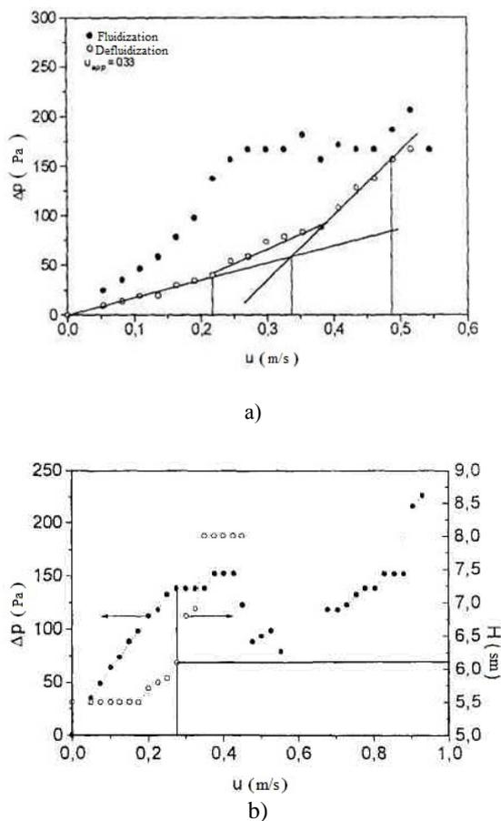
Fig 4. Curves for fluidization of a bed consisting of particles obtained by: (a) crushing of furniture fittings, (b) crushing of wooden structures
