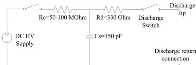
Fig. 2 Simplified diagram of the ESD generator [1]
