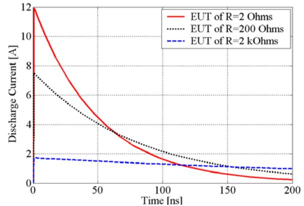
Fig. 3 Current waveforms from the PSpice program for the RC circuit with an ohmic EUT [11]
