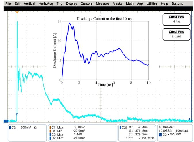
Fig. 5 Current waveform taken by the oscilloscope TDS 7254B for a charging voltage of + 4 kV. The first 10 ns of the ESD are presented in detail at the upper right part of the figure current
