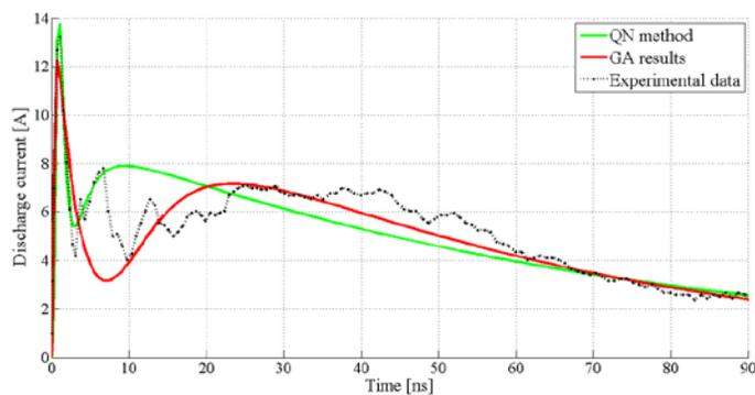
Fig. 7 Comparison between the experimental data of the electrostatic discharge current and the electrostatic discharge current for the optimized parameter values obtained from the genetic algorithm (GA) and the quasi-Newton (QN) optimization algorithm (charging voltage = + 4 kV)
