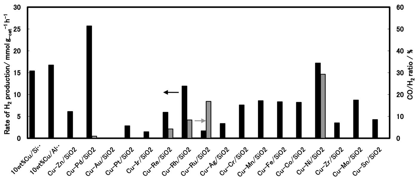
Fig. 2 Rate of H<sub>2</sub> production and CO/H<sub>2</sub> ratio in products of methanol-steam reforming over some Cu/SiO<sub>2</sub> catalysts prepared by using the sol-gel method at 200 °C. Catalyst weight: 0.1 g, CH<sub>3</sub>OH-H<sub>2</sub>O = 16-16 mmol g<sub>cat</sub><sup>-1</sup> h<sup>-1</sup>.
