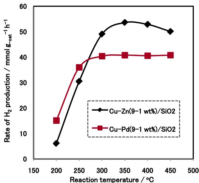
Fig. 3 Reaction temperature dependence of H<sub>2</sub> production rate of methanol steam reforming over Cu-Zn(9-1 wt%)/SiO<sub>2</sub> catalyst and Cu-Pd(9-1 wt%)/SiO<sub>2</sub> catalyst prepared by using sol-gel method. Catalyst weight: 0.1 g, CH<sub>3</sub>OH-H<sub>2</sub>O = 16-16 mmol g<sub>cat</sub><sup>-1</sup> h<sup>-1</sup>.
