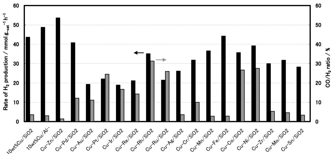
Fig. 1 Rate of H<sub>2</sub> production and CO/H<sub>2</sub> ratio in products of methanol-steam reforming over some Cu/SiO<sub>2</sub> catalysts prepared by using the sol-gel method at 350 °C. Catalyst weight: 0.1 g, CH<sub>3</sub>OH-H<sub>2</sub>O = 16-16 mmol g<sub>cat</sub><sup>-1</sup> h<sup>-1</sup>.
