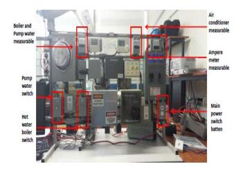
Fig 3. The represented the Smart Grid platform in HIT Forward view
