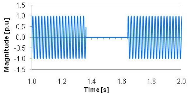
Fig. 9 Incidence of interruption in voltage signal
