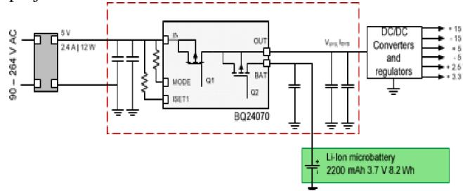
Fig. 6 Schematic of redundant power supply
