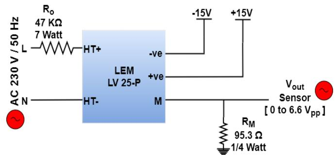
Fig. 2 Schematic of Voltage Sensor
