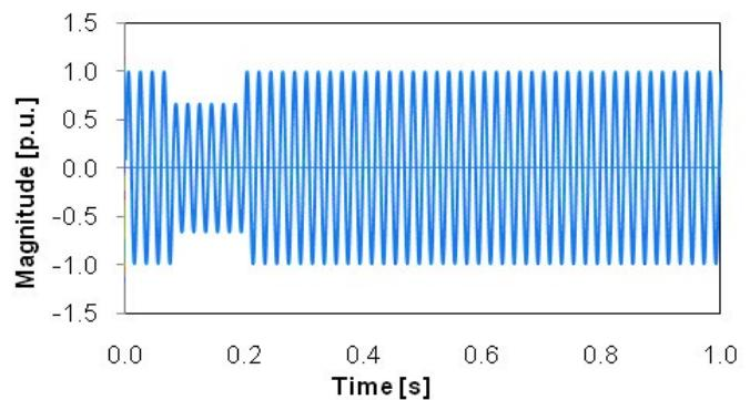
Fig. 14 Incidence of sag in voltage signal
