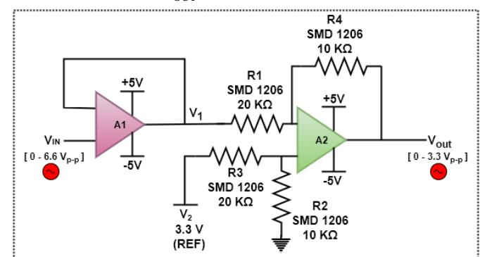
Fig. 3 Schematic of signal conditioning circuit
