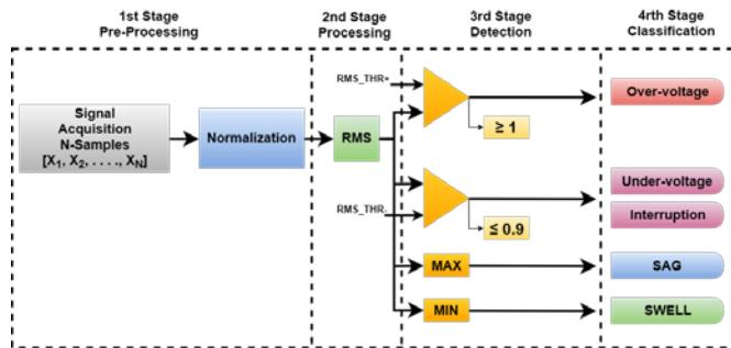
Fig. 7 Block diagram of different stages
