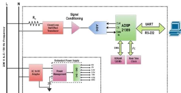
Fig. 1 Block diagram of PQ analyzer
