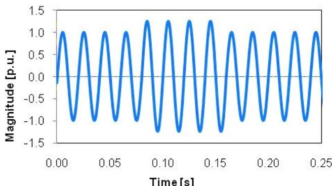
Fig. 12 Incidence of swell in voltage signal (detail)
