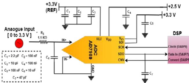
Fig. 4 Schematic of the A/D converter
