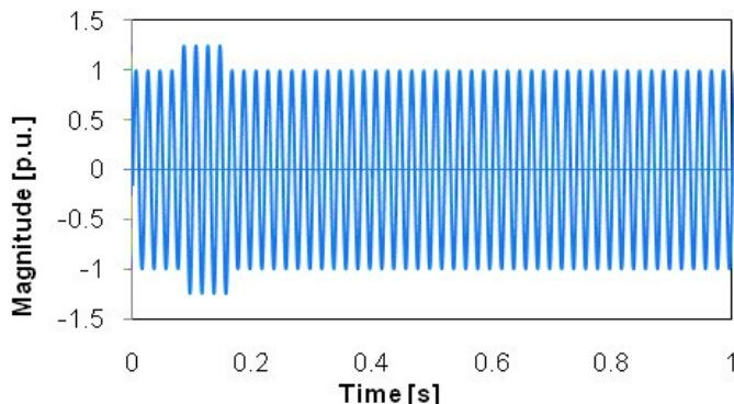
Fig. 11 Incidence of swell in voltage signal
