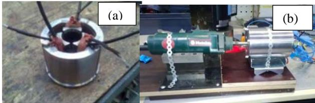
Figure 7(a) CNT windings used in the stator of a 3 tooth 2 pole motor (b) The motor is connected back to back with a commercially available commutator motor grinding machine to act as a generator.[33][Reproduced by permission of Praize Worthy Prize S.R.L]
