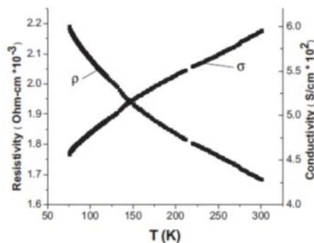
Figure. 2. Temperature dependence of the resistivity ( $\rho$ ) and conductivity ( $\sigma$ ) of a spun CNT fiber [14] [Image reproduced by permission of John Wiley & Sons].
