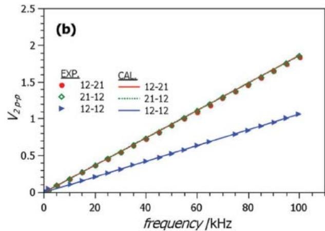
Figure 6(a) Illustration of the windings used for conducting the experiment (b) Output voltage across the secondary as a function of frequency. [32] [Image reproduced by permission of John Wiley & sons]
