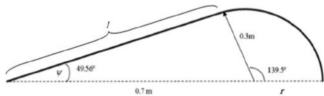
Figure 4 – Optimized Profile Configuration
