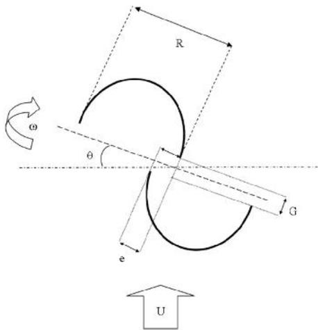
Figure 1- Typical Savonius rotor configuration
