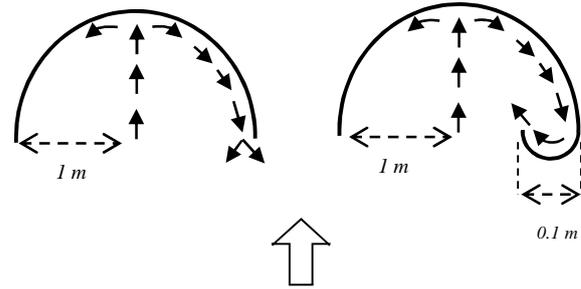
Figure 2- Left: Conventional Savonius rotor, Right: Savonius rotor with tip fin
