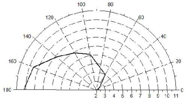
Figure 9- Effect of angle of tip device on performance of the rotor
