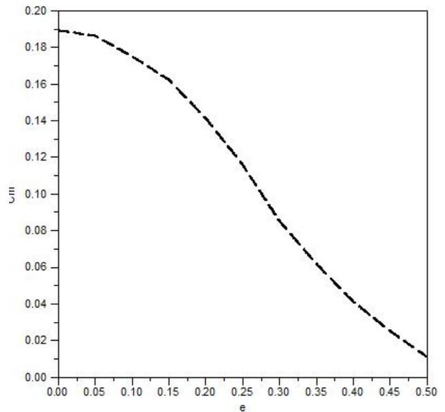
Figure 6- Effects of increment of overlap ratio on power coefficient
