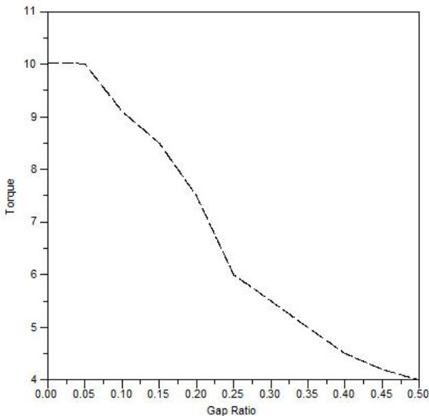
Fig.8 Effects of increment of overlap ration on output torque
