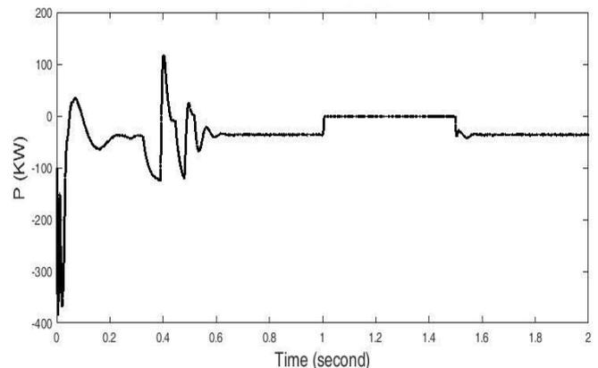
Fig.9. Power at the grid terminal with Load (120kw)
