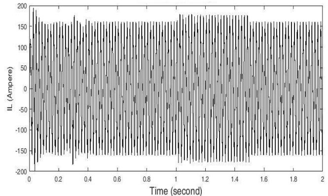
Fig.8. Current at load terminal (70kw)
