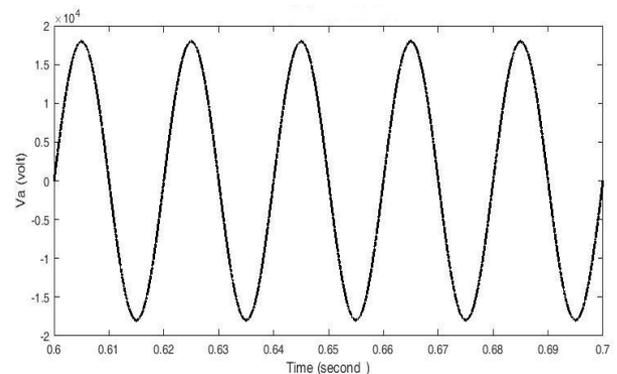
Fig.3.  $V_a$  at the grid terminal
