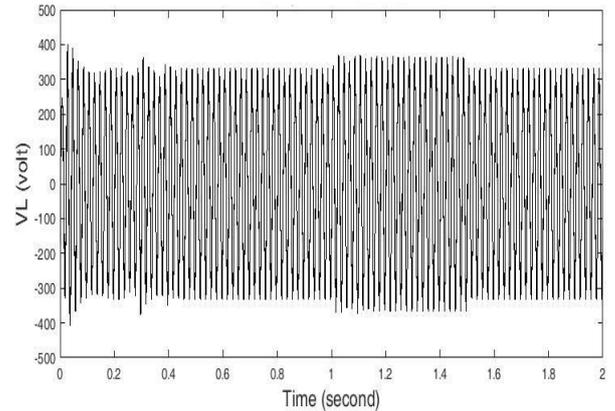
Fig.7 Voltage at load terminal (70kw)
