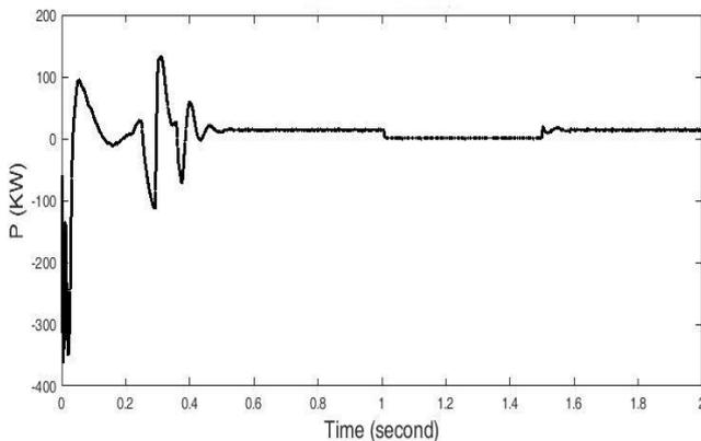
Fig.5. Power at the grid terminal with Load (70kw)
