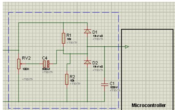
**Figure 3: A-V Measurement Circuit**
