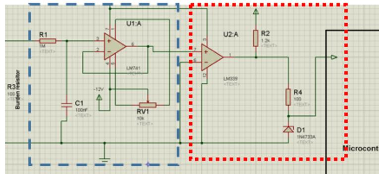
**Figure 4: Power Factor Measurement Circuit**
