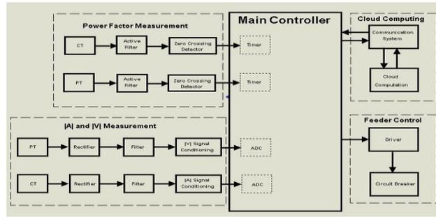
**Figure 1: Overall block diagram for the monitoring and fault detection system**
