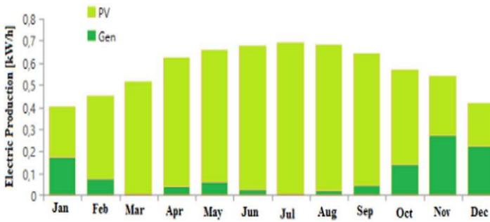
Fig.5 Average monthly electricity production from Solar PV's and diesel generators
