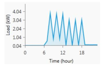
Fig. 2 Typical daily load profile for cement bricks factory
