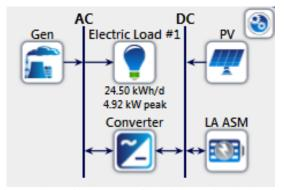
Fig.3 Schematic diagram of hybrid PV-diesel - battery system
