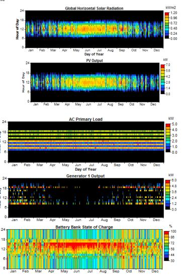
Fig. 8 Power production of different power sources and battery SOC
