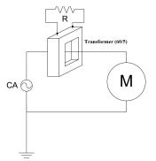
Fig.4. Measuring the current of the motor
