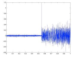
Fig. 7. Coefficient of details using wavelet of Haar level 1
