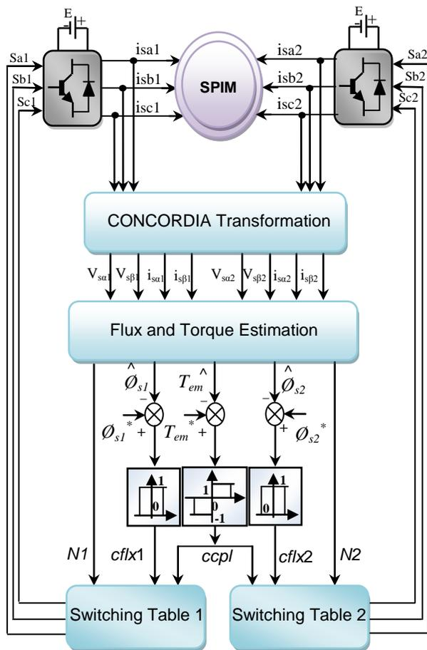
Fig. 3 Block diagram of Direct Torque Control for SPIM
