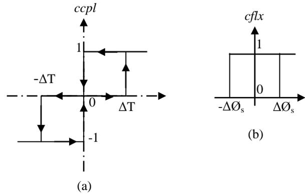
Fig. 4 Hysteresis comparator, (a): three level hysteresis comparator for the torque, (b): two level hysteresis comparator for the flux
