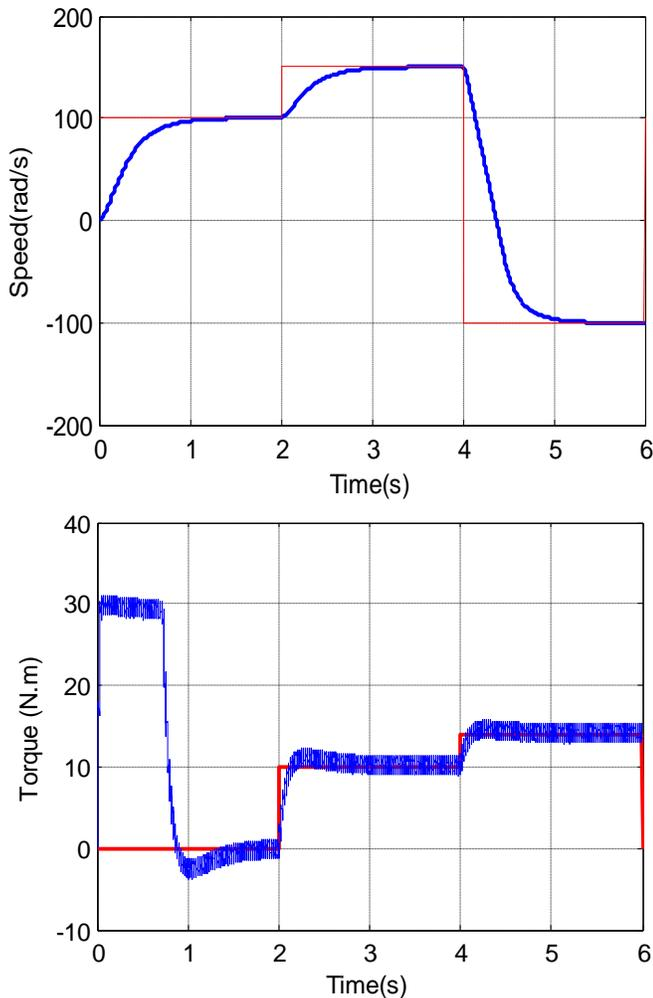
Fig. 8 DTC of SPIM with speed and load variation
