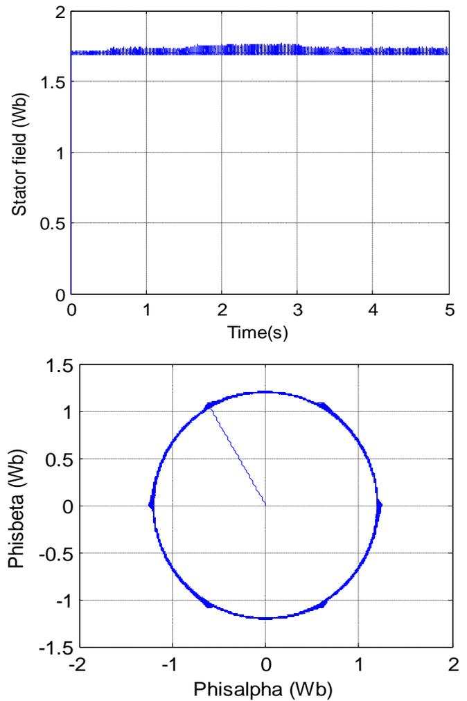
Fig. 7 DTC of SPIM with load torque (14 N.m) between [1.5 3] s
