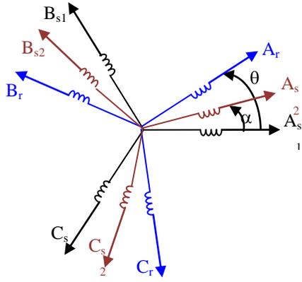
Fig. 1 Windings of the Six Phase Induction Machine
