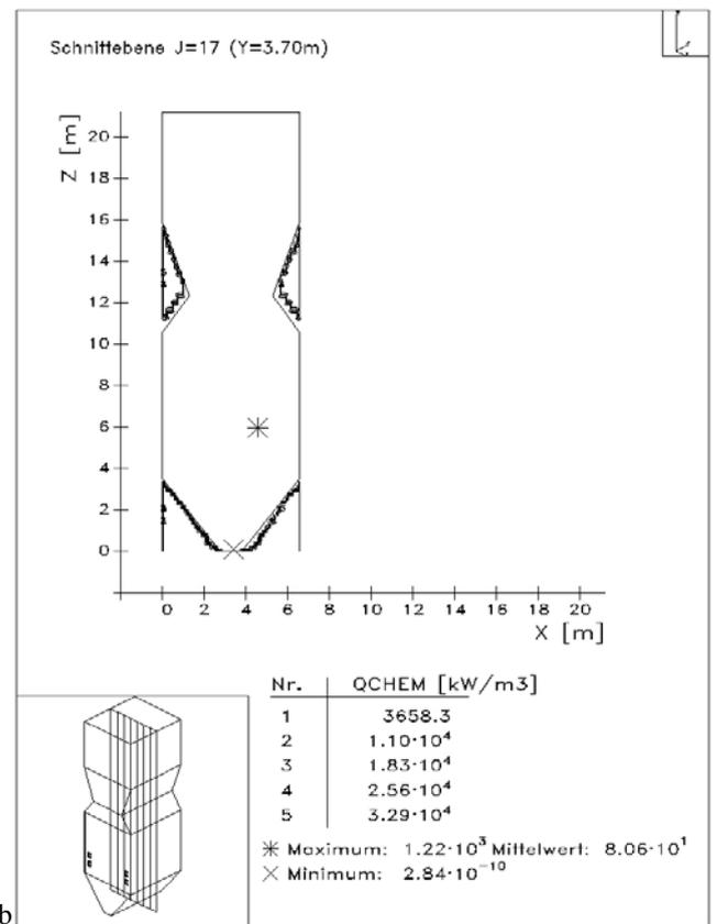
Fig. 11. (a, b) – Isosurfaces of energy distribution of chemical reaction
