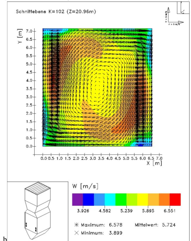
Fig. 9. (a, b) – Distribution of V-component of the vector of full speed in the burner section and in upper section of investigated combustion chamber
