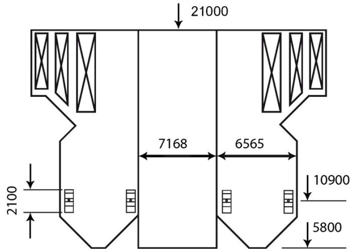
Fig. 3. Layout of the combustion chamber of the boiler BKZ-160
