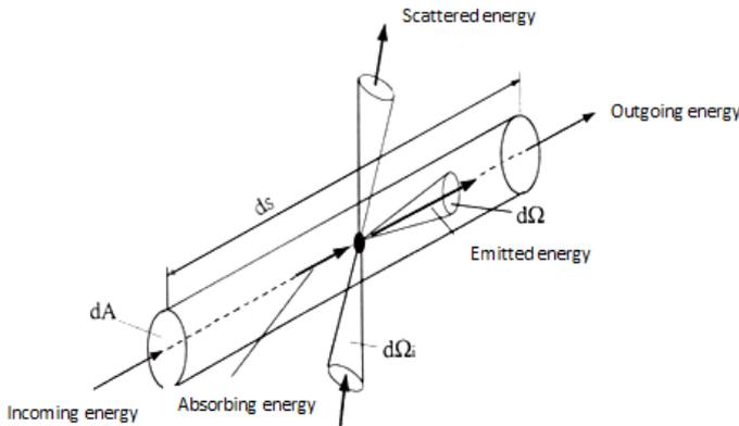
Fig. 2. Change of intensity along the element  $ds$
