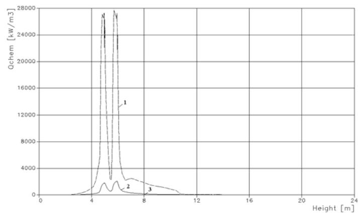
Fig. 12. The distribution of chemical energy  $Q_{chem}$  by the height of the combustion chamber
