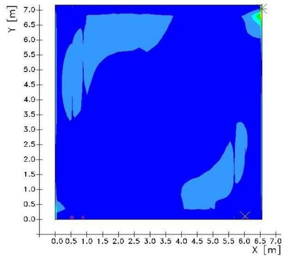
Fig. 14. The distribution of chemical energy  $Q_{chem}$  at the outlet of the combustion chamber
