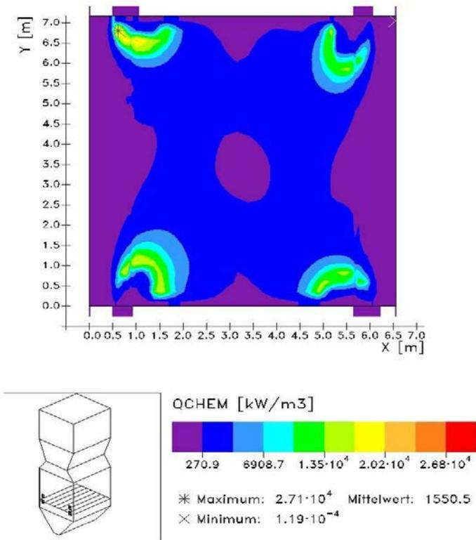
Fig. 13. The distribution of the chemical energy  $Q_{chem}$  in cross section of combustion chamber at the lower tier of burners
