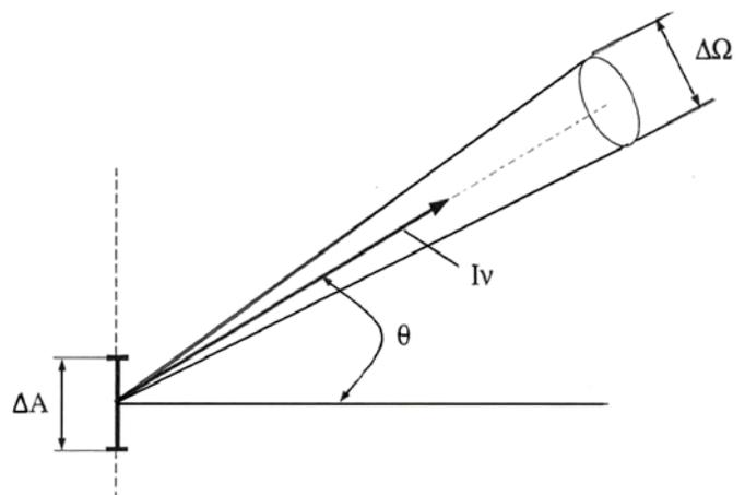
Fig. 1. Determination of the spectral intensity
