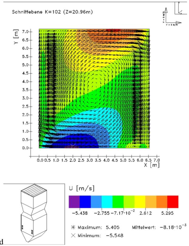
Fig. 8. (a, b, c, d) – Distribution of U-component of the vector of full speed in different sections of the investigated sections of combustion chamber
