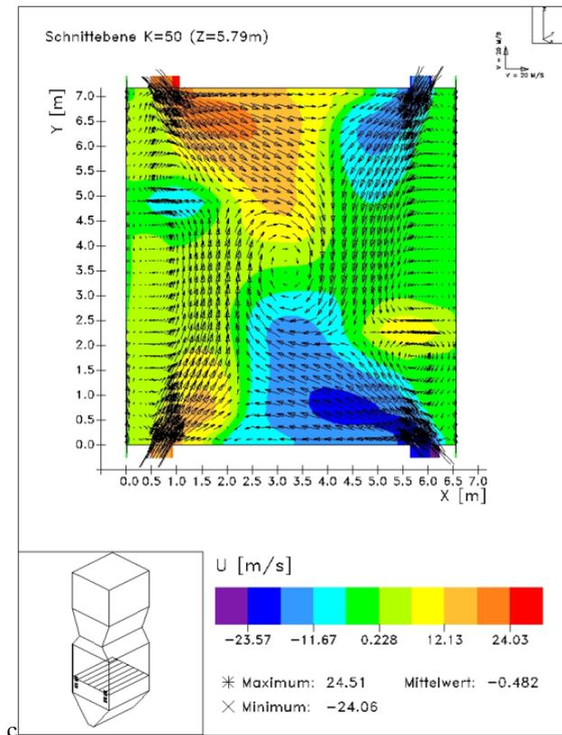
Figure 8 clearly shows the aerodynamic flow pattern of a mixture of pulverized coal flow through the tangential burner.
