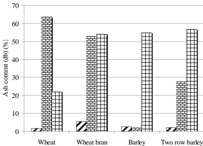
Fig. 7 Variation of substrate ash content during anaerobic digestion process: 0 - /, 40 - #, 65 - #
