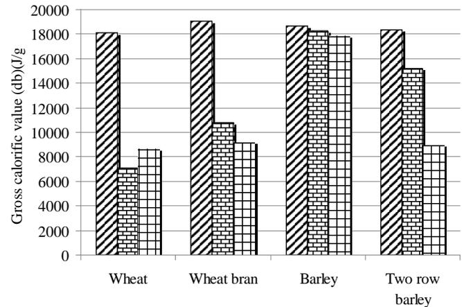
Fig. 8 Variation of substrate gross calorific value during anaerobic digestion process: 0 - /, 40 - #, 65 - #
