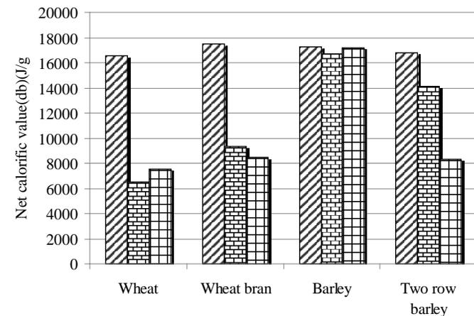
Fig. 9 Variation of substrate net calorific value during anaerobic digestion process: 0 - /, 40 - #, 65 - #
