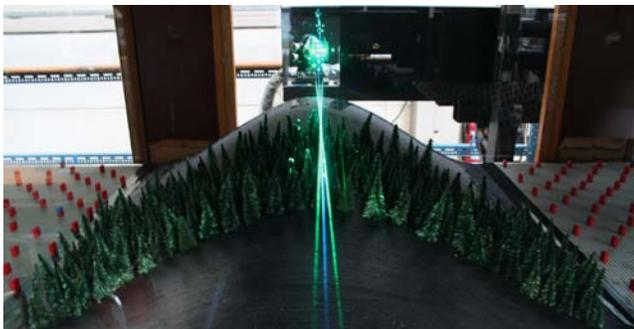
Fig. 2: 2D-LDA system for flow measurements
