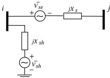
Fig. 2. Equivalent model of UPFC.
