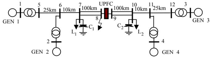
Fig. 10. A simple two-area power system model.
