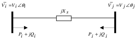
Fig. 7: Injection model of the series part of the UPFC
