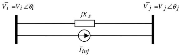
Fig. 6: Transformed series voltage source
