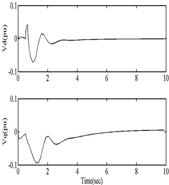
Fig. 13: series injected voltage by UPFC for damping oscillations.
