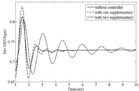
Fig. 17: Active power oscillation of GEN3 to three phase fault with one and two supplementary damping signals
