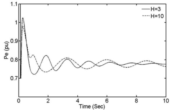
Fig. 11: Response of test power system to changes of inertia coefficient of generators.
