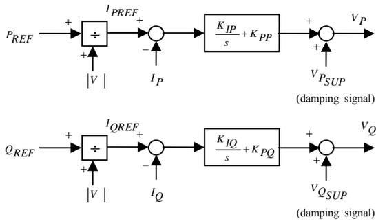
Figure 9: the series part of the control system of UPFC
