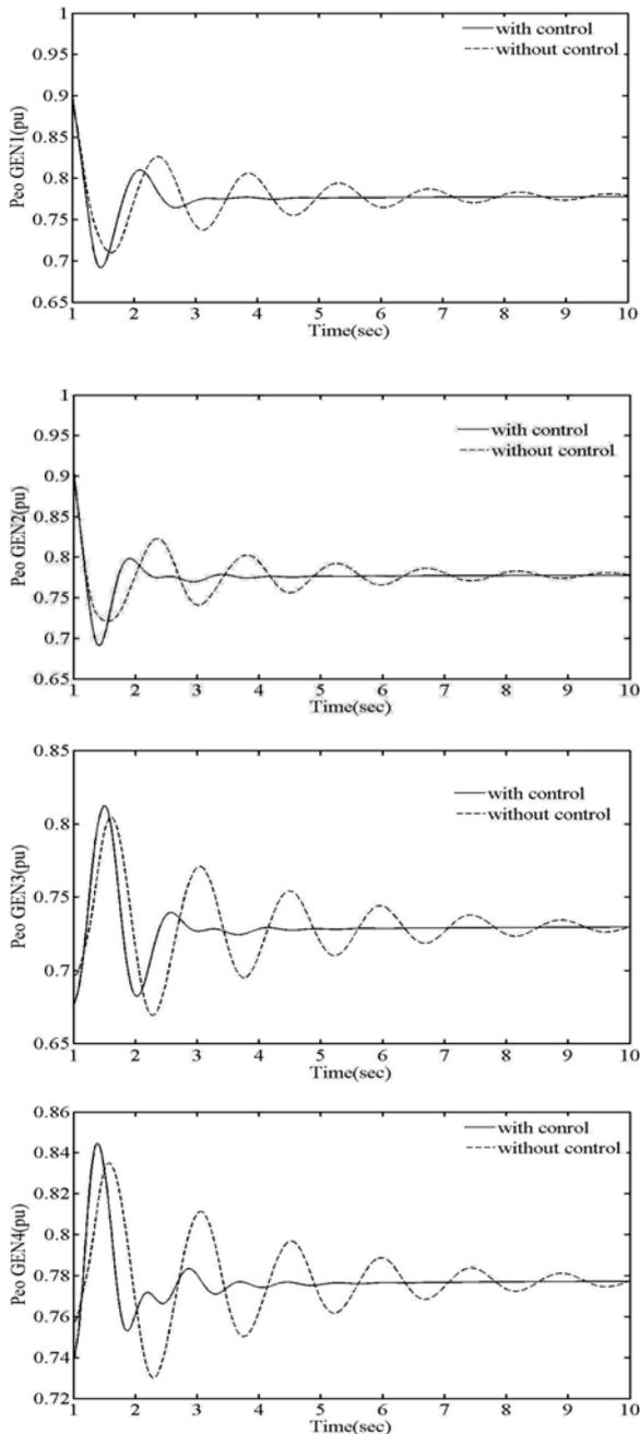
Fig. 15: Active power oscillation of generators to three phase fault with and without controller.
