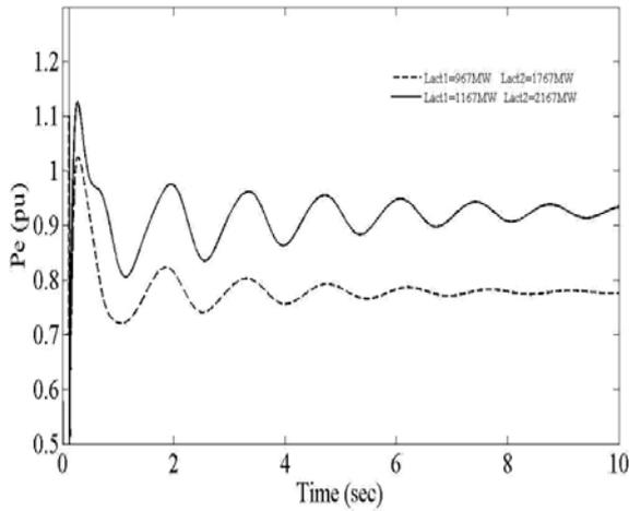
Fig. 12: Response of test power system to changes of active loads
