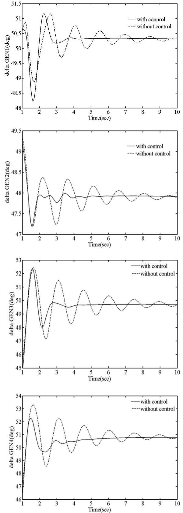
Fig. 14: Machine angle oscillation of generators to three phase fault with and without controller.
