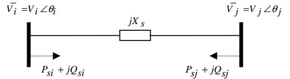
Fig. 8: Injection model of the UPFC
