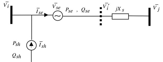
Fig. 3: Equivalent circuit diagram of UPFC
