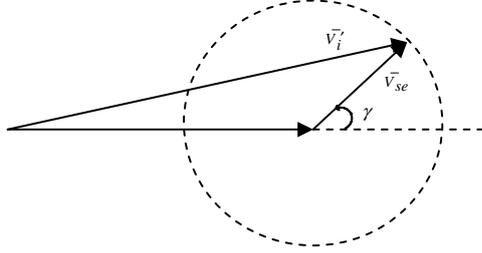
Fig. 4: Vector diagram of the equivalent circuit of series voltage source
