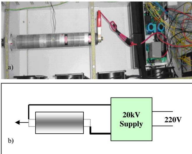
Fig. 3 (a) Top view of the laser system (b) 20 kV power supply connected to CO<sub>2</sub> laser tube terminal
