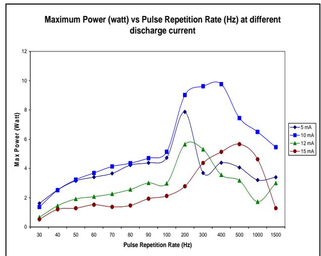
Fig.9. Maximum power as function of pulse repetition rate at different discharge current
