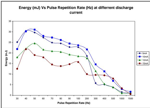
Fig.7 Output pulse energy as a function of pulse repetition rate at different discharge current
