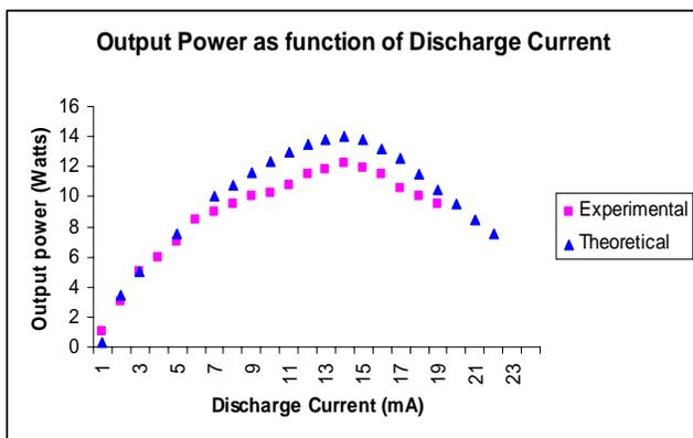
Fig.12 Calculated and Measured Output Power as Function of Discharge Current
