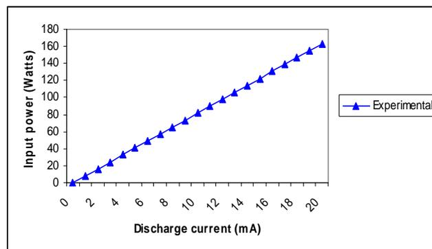
Fig.6. Input power as function of Discharge current
