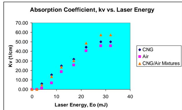
Fig.13 Absorption coefficient,  $k_v$ , of CO<sub>2</sub> laser in CNG, air and CNG/Air mixtures on the initial laser energy,  $E_0$
