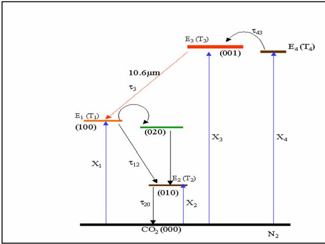
Fig.1 energy level diagram of lasing mechanism in CO<sub>2</sub> laser [5-7]
