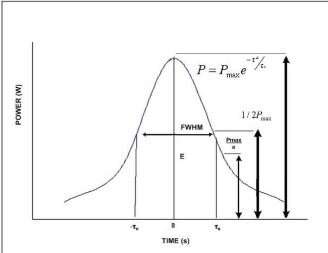
Fig.2 Gaussian distribution from a single pulse of laser power [10]
