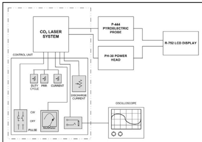
Fig.4 Block Diagram for Measurement of Output Parameters of CO<sub>2</sub> Laser.
