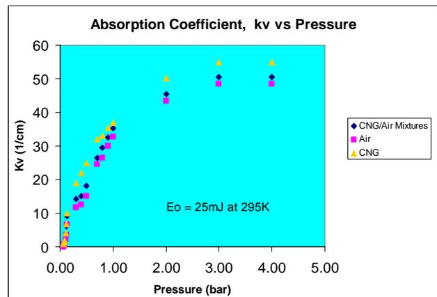
Fig.14 Absorption coefficient,  $k_v$ , of CO<sub>2</sub> laser in CNG, air and CNG/Air mixtures on gases pressure
