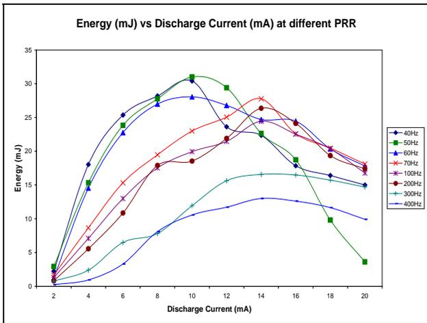
Fig.8 Output pulse energy as a function of discharge current at different pulse repetition rate
