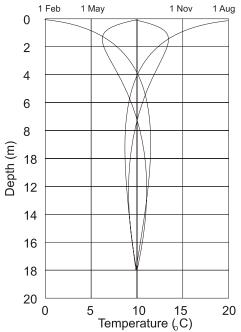
Fig. 5 range of temperatures in the Earth over the year depending on depth [5], [6]
