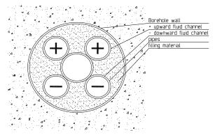
Fig. 3 schematic cross section of typical Double U-pipe BHE [7]
