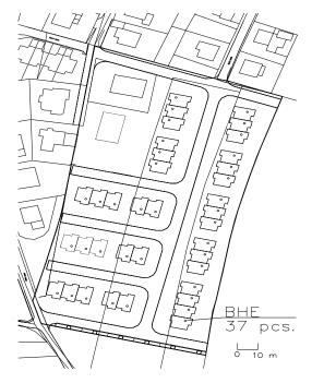
Fig. 1 proposition of BHE arrangement for residential area project
