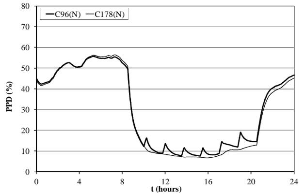
Fig.34 – PPD index numerically obtained in two compartments turned to north, for a typical winter day.
