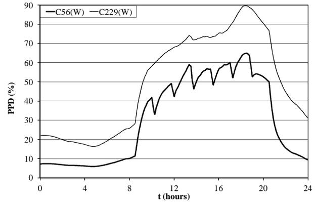
Fig.33 – PPD index numerically obtained in two compartments turned to west, for a typical summer day.
