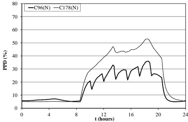
Fig.30 – PPD index numerically obtained in two compartments turned to north, for a typical summer day.
