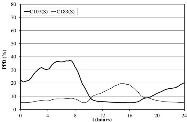
Fig.27 – PPD index numerically obtained in two compartments turned to south, for a typical winter day.
