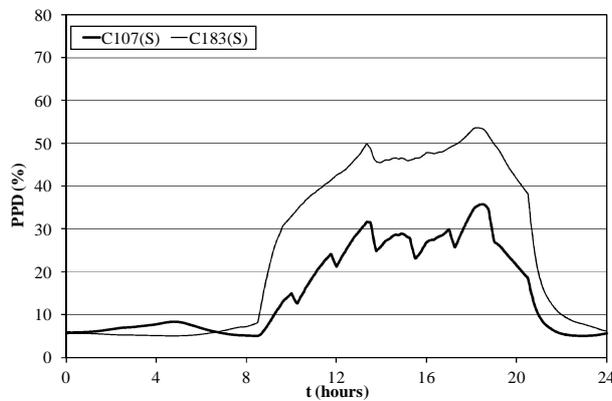
Fig.31 – PPD index numerically obtained in two compartments turned to south, for a typical summer day.
