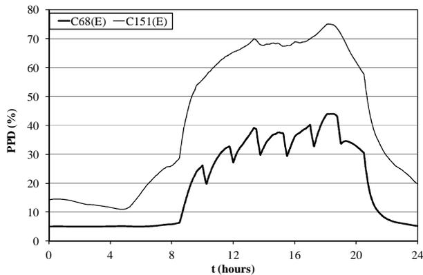
Fig.32 – PPD index numerically obtained in two compartments turned to east, for a typical summer day.
