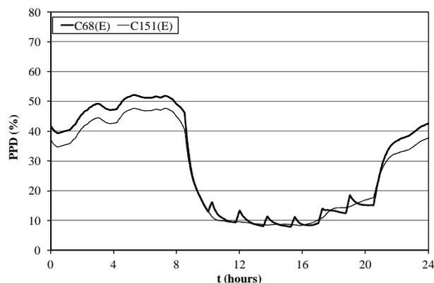
Fig.36 – PPD index numerically obtained in two compartments turned to east, for a typical winter day.
