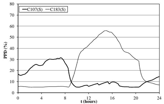
Fig.35 – PPD index numerically obtained in two compartments turned to south, for a typical winter day.
