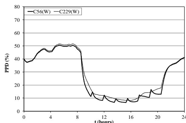
Fig.37 – PPD index numerically obtained in two compartments turned to west, for a typical winter day.
