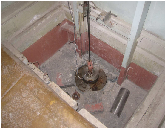
Fig.4 Samples are irradiated in ^{60}\text{Co} Isotopic Radiation Source
