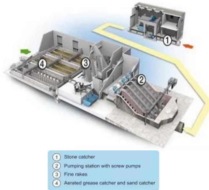
Fig. 3: Process of mechanical treatment [8]
