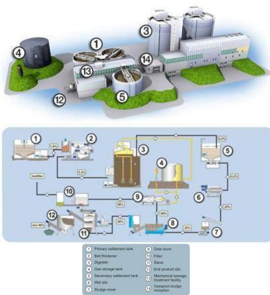
Fig 5: Anaerobic process biological treatment of wastewater [8]
