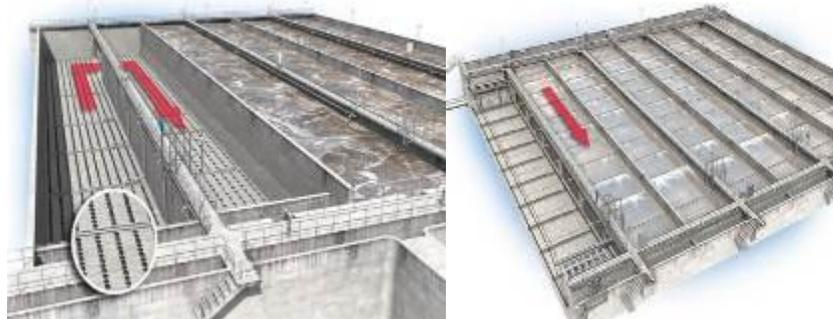
Fig 4: Aerobic process of biological wastewater treatment [8]
