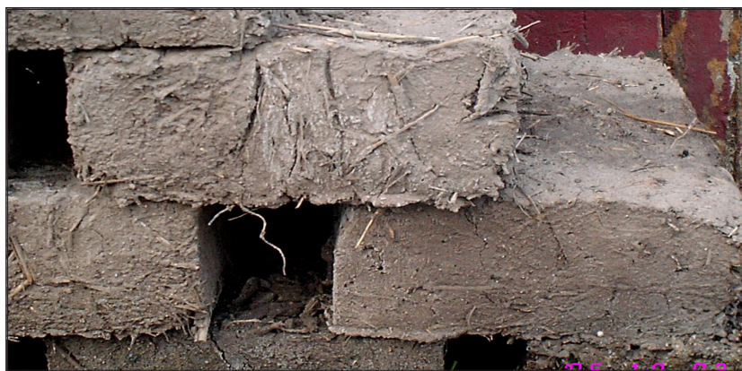
Figure 5: Contemporary adobe bricks exposed for drying in open air in the yard of a local.
