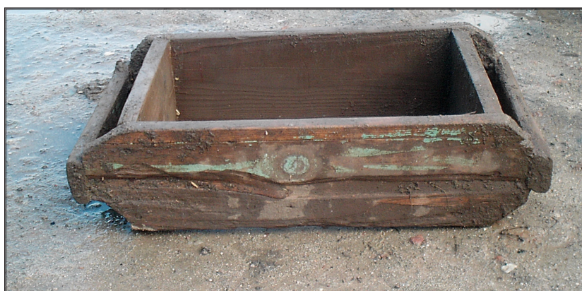
Figure 6: Contemporary wooden mold for formatting adobe bricks. Utensil used by the same local.
