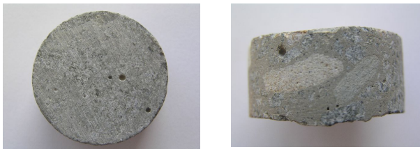
Fig. 1: Concrete samples prepared for corrosion experiment
