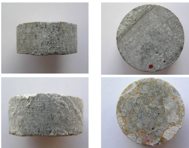
Fig. 5: Concrete samples before and after corrosion experiment (immersed into the H_2SO_4 )
