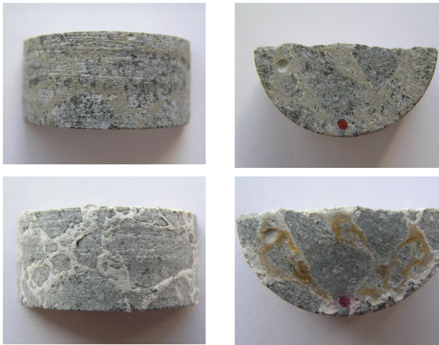
Fig. 4: Concrete samples before and after corrosion experiment (immersed into the H_2SO_4 )
